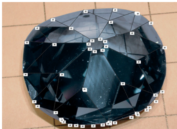
Figure 4. Facet junctions were labeled so their locations could be plotted during photo analysis. Photo by S. W. Attaway.
