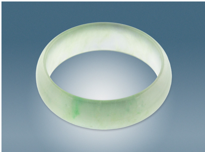
Figure 15. The remarkable transparency of this jadeite bangle is due to impregnation with a polymer that has an RI very close to that of the host material.
