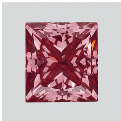
Figure 13. This 0.74 ct Fancy red diamond ( 4.85 \times 4.41 \times 3.67 mm) was identified as a CVD synthetic. Multiple treatments were applied after the initial growth to produce this color.
