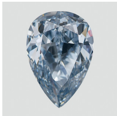
Figure 8. This 6.46 ct Fancy Intense blue diamond is one of the largest HPHT-treated type IIb diamonds seen in the GIA lab.
