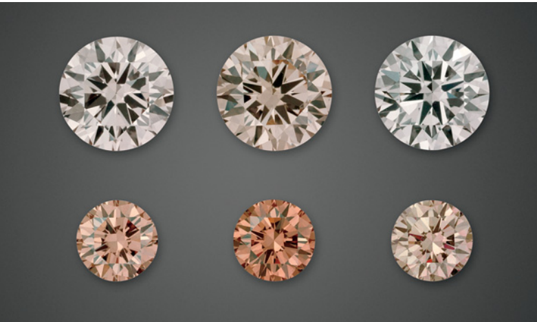
Figure 2. These images illustrate samples 3 (top; 0.92 ct) and 5 (bottom; 0.40 ct) in their initial (stable) states (left), after UV exposure (center), and after heating (right). Composite photo by R. Khan.
