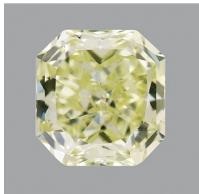
Figure 10. The greenish yellow color of this 0.90 ct type IIa diamond is caused by an IR-inactive nitrogen-related defect.
