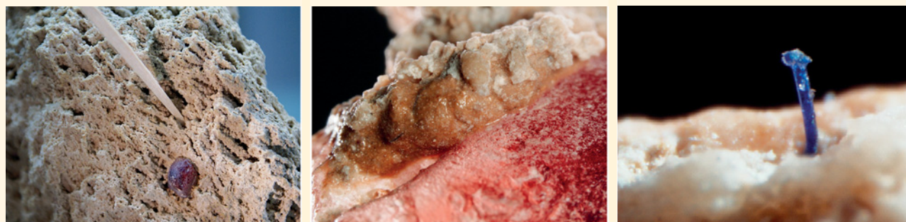
Figure 8. The matrix samples contained rounded pieces of andesine embedded in porous carbonate rock that had the appearance of caliche (e.g., left image). The junction of the andesine and the matrix, as well as the surrounding area, contained a material that made the porosity of the matrix look wet and shiny (center, field of view 4.0 mm). One specimen contained transparent blue fibers that were flexible (right, field of view 1.0 mm) and partially melted during Raman analysis, which produced spectra similar to nylon. Photos by K. Scarratt (left) and S. F. McClure.
