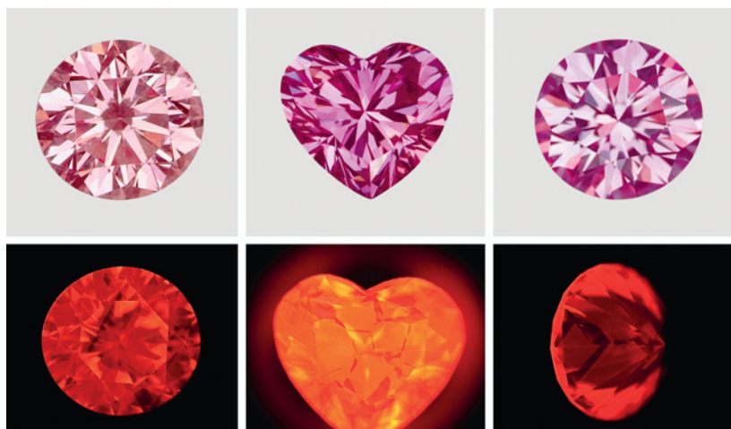
These three synthetic diamonds (0.14, 0.20, and 0.53 ct) owe their coloration to a combination of carefully controlled growth and treatment. Subtle growth structures are visible in their corresponding DiamondView images. Photos by Jian Xin (Jae) Liao (top), K. S. Moe (bottom left and right), and P. Johnson (bottom center).
