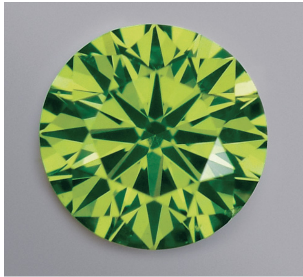
This 0.24 ct diamond was treated by multiple processes, including HPHT annealing and irradiation, to achieve its attractive Fancy Intense yellowish green color. Photo by C. D. Mengason.
