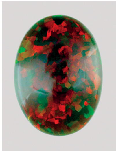
Figure 13. This 10.67 ct opal cabochon is reportedly from the Wollo Province of Ethiopia. The black bodycolor is caused by natural manganese oxides incorporated during formation.
