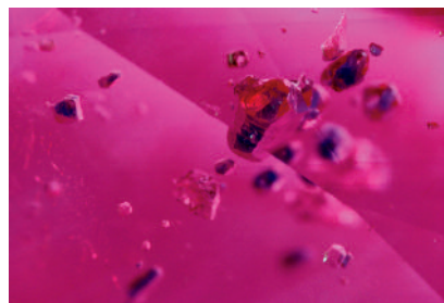
Figure 14. A 5.09 ct ruby was host to numerous lazurite-filled negative crystals. Magnified 25 \times .
