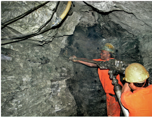
Figure 4. At Montebello, miners drill into the hard schist to prepare it for blasting. Photo by A. Lucas.
