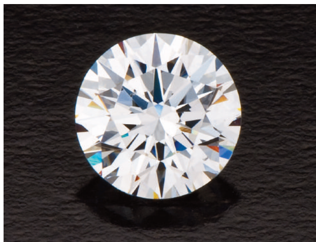
Figure 1. This cubic zirconia (2.00 ct) has been coated by Serenity Technologies with a proprietary colorless thin layer that is said to consist of “nanocrystalline diamond particles” embedded in a matrix. Photo by Robert Weldon.
