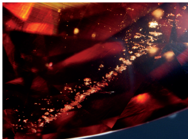
Figure 35. Microscopic observation of the spessartine revealed whitish irregularly shaped corroded inclusions. Photomicrograph by HyeJin Jang-Green; field of view 3.0 mm.
