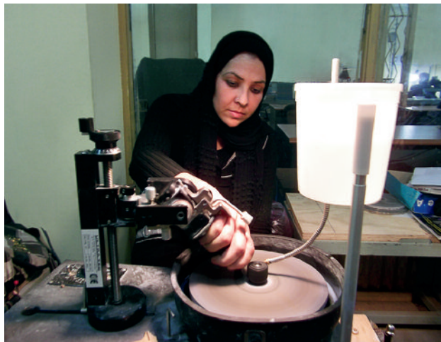
Figure 17. An Afghan woman in Kabul facets with a modern Ultra Tec machine. Photo by Jim Rentfrow.
