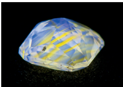
Figure 6. When the diamond was exposed to long-wave UV radiation, the orange-yellow color zones fluoresced very strong yellow-orange, while the near-colorless zones showed strong blue fluorescence.
