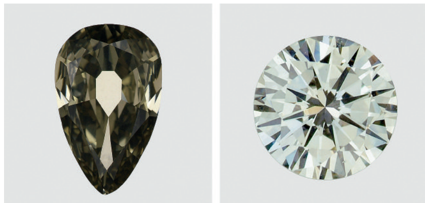
Figure 2. These type IIb samples consist of a Fancy Dark gray-yellowish green natural diamond (5.84 ct, left) and a Fancy Light yellow-green synthetic diamond (0.30 ct, right).
