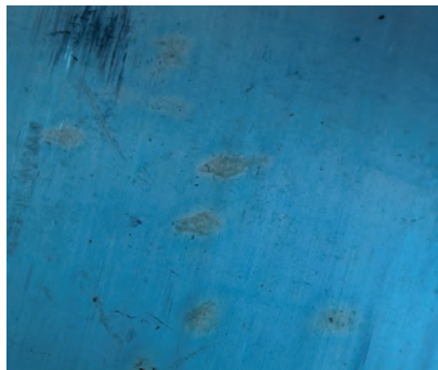
Figure 6. Decolorized areas corresponding to surface damage confirmed that the blue color of the gypsum cabochon resulted from the thin coating, which was identified as a polymer resin by Raman spectroscopy. Image width: 4.3 mm.
