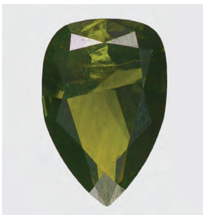
Figure 1. This 2.34 ct Fancy Deep yellow-green diamond was identified as artificially irradiated and annealed. The green color is predominantly due to the H2 defect, an extremely rare occurrence.
