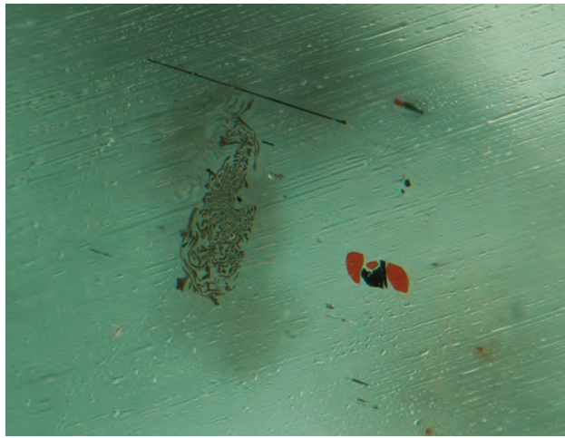
Figure 3. A variety of inclusions were identified in the Malagasy aquamarine. Shown here are platelets composed of reddish brown hematite and black ilmenite, as well as dark gray dendritic inclusions and black needles of ilmenite. Photomicrograph by V. Bourgoïn; image width 1.0 mm.
