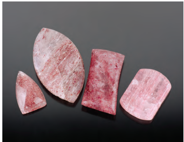
Figure 30. These quartz cabochons (18.57–61.06 ct) from central Tanzania contain bright red inclusions of a mineral in the epidote-piemontite series. Photo by Robert Weldon.
