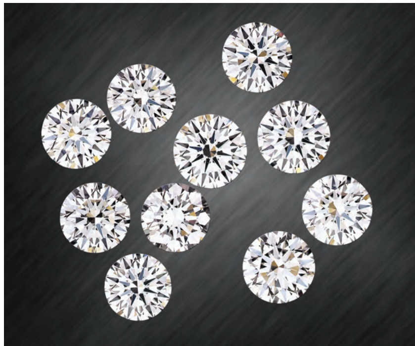
Figure 10. These 10 CVD synthetic diamonds (0.30–0.35 ct, with F–H color) were recently identified in GIA's Hong Kong laboratory.
