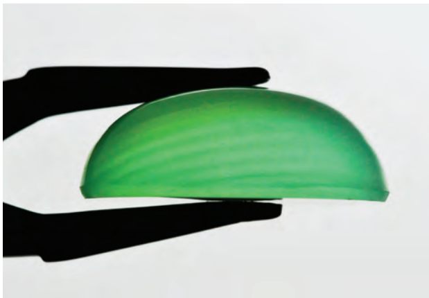
Figure 5. In certain directions, the calcites displayed banding along their length, indicating layered growth. The pattern was readily apparent in the green sample but more subtle in the orangy yellow stone. Photo by G. Choudhary.
