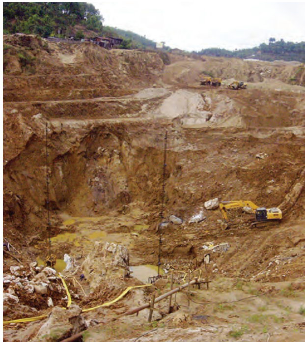
Figure 18. This open pit at Ingaung is a source of ruby and sapphire, which are mined from secondary deposits. Photo by U T. Hlaing.
