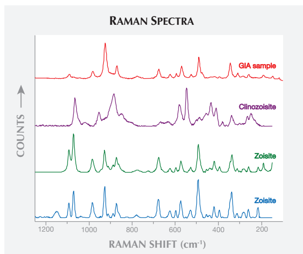
Figure 35. The Raman spectrum of the 3.14 ct sample from Pakistan show the best match to the reference spectra for zoisite rather than clinozoisite.
