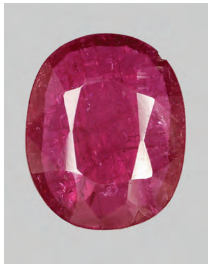
Figure 14. This 11.52 ct synthetic ruby proved to be filled with lead glass.
