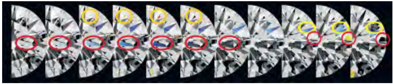
Figure 25. Each image shows a 2° rotation clockwise from the previous image. A spot light source contributes a small amount of fire (seen here as red, blue, green, or yellow virtual facets). As the gem is rotated, some virtual facets go from light to dark (examples are circled). As a facet nears the border between light and dark, the observer will see fire. Some of these flares of color last through larger degrees of rotation than others (larger red circles). While not illustrated, when a facet only slightly darkens or lightens, fire is faint. Strong changes in contrast create stronger fire. More fire is exhibited by materials of higher dispersion values.
