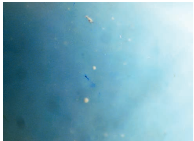
Figure 13. Microscopic observation reveals dark blue color concentrations and whitish gas bubbles. Photomicrograph by Lore Kiefert; magnified 40 \times .
