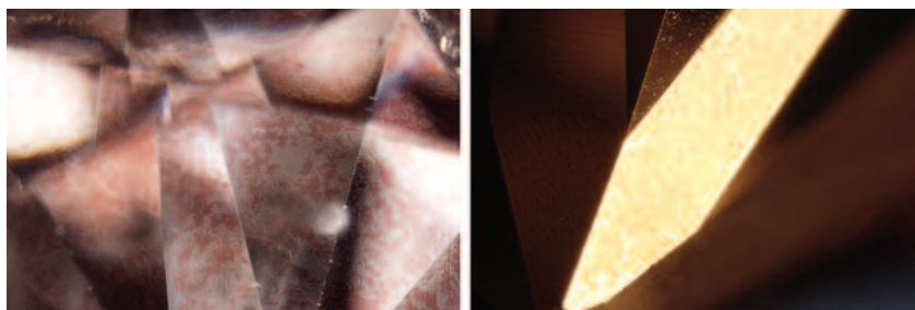
Figure 5. Photomicrographs of the diamonds from figure 4, taken with reflected light at 80× and 100× magnification, reveal the coating applied to the pavilion facets.
