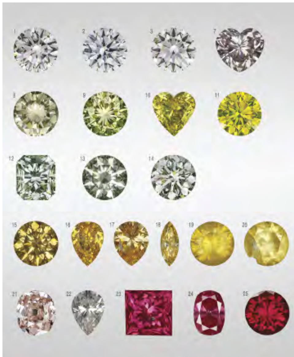
Figure 5. Diamonds with N3 defect centers include samples 1–3, which are colorless (1 and 3 have a brownish hue); samples 4–6, which are near colorless to faint yellow (not shown); and sample 7, a pink diamond with both N3 and H3 defect centers. Samples with the H3 center (8–11) and H4 center (12–14) are yellow to light green. Diamonds with the 480 nm band (15–20) are yellow to orange, while those with N-V centers (21–25) are pale to intense pink or red. Photos by Don Mengason and Robison McMurtry.
