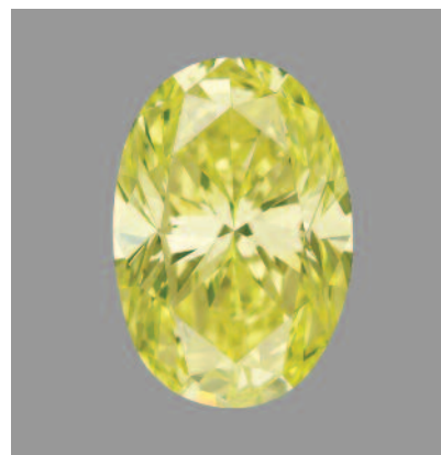
Figure 7. This 24.16 ct oval-cut diamond (20.47 × 14.00 × 10.72 mm) was color graded as Fancy Intense green-yellow, and identified as artificially irradiated and annealed.
