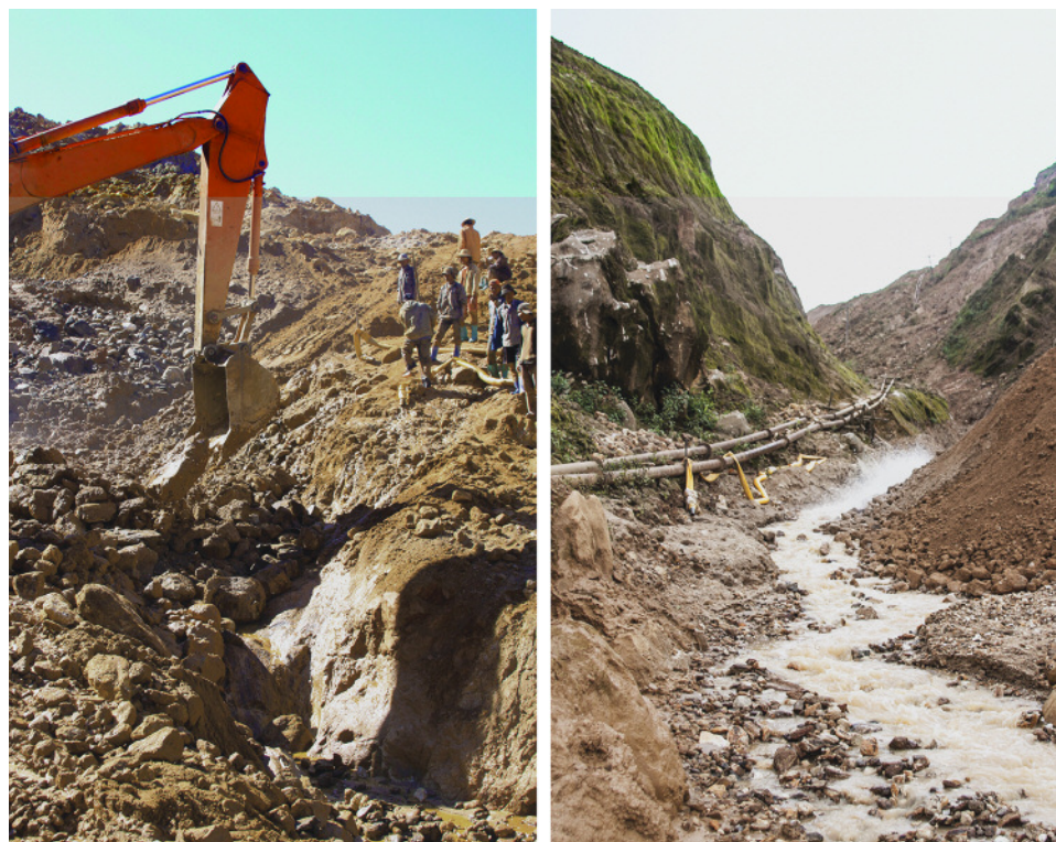
Figure 6. Left: Miners use excavators to remove gem-bearing overburden gravels. Right: The gravels are transported downstream to the washing plant using water supplied by the pipes. Photos by Hpone-Phyo Kan-Nyunt.
