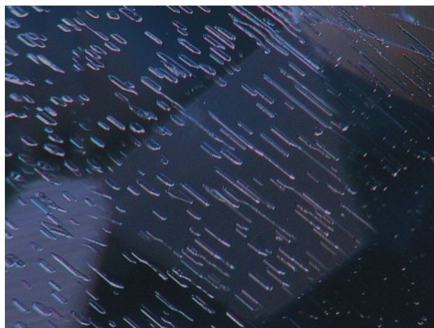
Figure 12. Healed fissure consisting of negative crystals in SABUM169. Photomicrograph by Hpone-Phyo Kan-Nyunt; magnified 25 \times .
