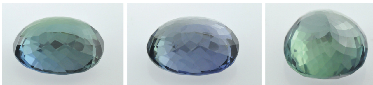
Figure 6. The artificially irradiated greenish blue spodumene displayed strong pleochroism, exhibiting three colors: blue (left), violet (center), and green (right). Photos by Gagan Choudhary.
