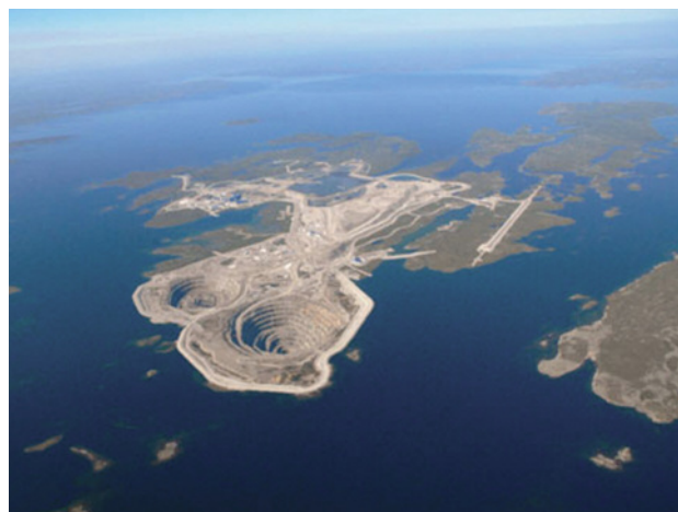
Figure 14. This aerial view shows the open pits containing the kimberlite pipes that comprise the bulk of the Diavik mine. The open pits outline the vertical geologic form of a typical kimberlite eruption, though the pit shape is wider than the actual kimberlite so that the pit walls do not collapse. The lines on the inside of the pit walls are benches along which massive 100-ton ore trucks are driven. Photo courtesy of Diavik Diamond Mine.
