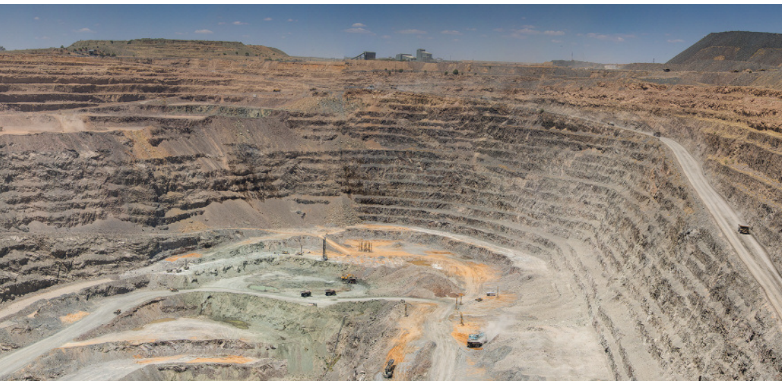
Figure 14. This panoramic view of the Jwaneng mine, Botswana's largest and most lucrative, shows a manmade pit—visible from outer space—that covers approximately 520,000 square meters at the surface and is more than 400 meters deep. Photo by Robert Weldon/GIA.
