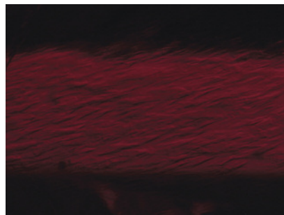
Figure 14. The zigzag-like growth structure observed in this 1.18 ct synthetic ruby is characteristic of hydrothermal growth. Field of view 1.42 mm.
