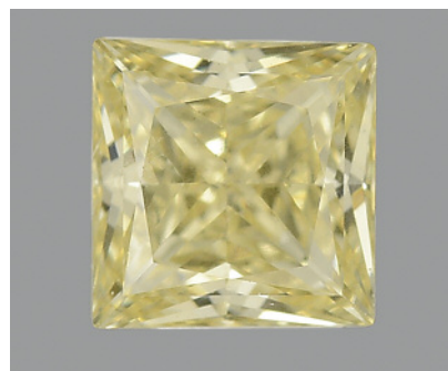
Figure 11. This 0.40 ct square-shaped type Ib CVD synthetic diamond was color graded as Fancy yellow.
