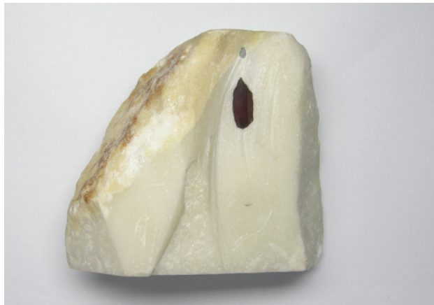
Figure 13. This synthetic ruby was fixed in a white and cream-colored matrix and represented as natural ruby. Photo by Sutas Singbamroong, Dubai Central Laboratory.
