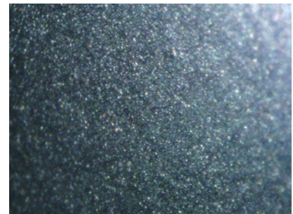
Figure 9. Top: The surface of the imitation pearls contained a glittery coating rather than overlapping nacre platelet structures (magnified 112.5 \times ). Bottom: White bead-like shell material was exposed at a damaged area near the drill hole (magnified 10 \times ).
