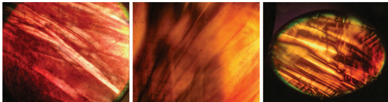
Figure 11. Microscopic features in Verneuil-grown diffusion-treated synthetic sapphires. Irregular grain boundaries are frequently observed under crossed polarizers (left and center); occasionally, glide planes (Plato lines) are also seen (right). Viewed in immersion; field of view: 8.1 \times 6.1 mm (left), 9.5 \times 7.2 mm (center), and 9.5 \times 7.2 mm (right). Photos by K. Schmetzer.
