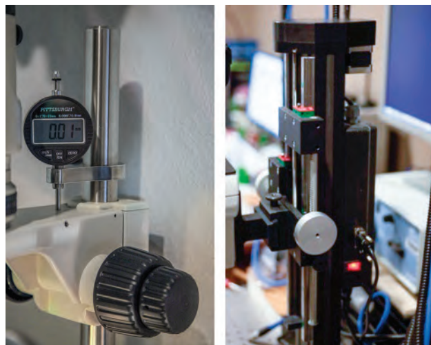
Figure 19. A digital indicator was attached to the author's microscope stand to accurately measure the step intervals for extended depth-of-field imaging. Left: The fine focus adjustment allows the microscope height to be precisely controlled to step intervals as small as 2.5 microns. Right: Sophisticated equipment such as this "Macrorail" can be used for automated image stacking when combined with the appropriate software. Photos by Nathan Renfro (left) and Darren Bates (right).
