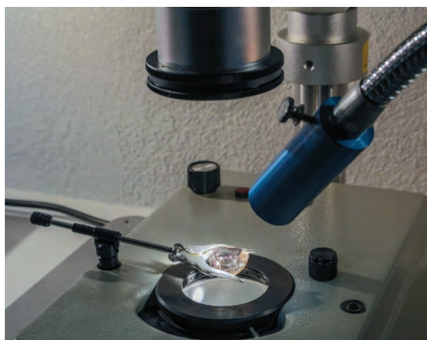
Figure 8. Oblique fiber-optic illumination can be used to reveal iridescent colors in reflective inclusions that might go otherwise unseen. Photo by Nathan Renfro.
