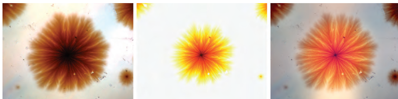
Figure 20. These radial manganese oxide "flowers" in Ethiopian opal provide too much contrast for the camera sensor to resolve all of the detail in the inclusion. The image at the left was underexposed, so detail is lost in the dark center of the MgO flower. The center image was overexposed to resolve detail in the dark areas, but all detail is lost in the bright areas. These varying exposure images were combined using HDR software (Nikon's NIS Elements) to produce the image on the right, which shows more detail than any single image. Photomicrographs by Nathan Renfro; field of view 2.47 mm.
