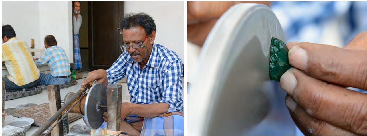
Figure 11. Tradition and skill outweigh technology at Green International, as these preformers prefer complete hand control over the emerald and the speed of the wheel for large free-size and calibrated stones. Photos by Andrew Lucas, courtesy of Green International.
