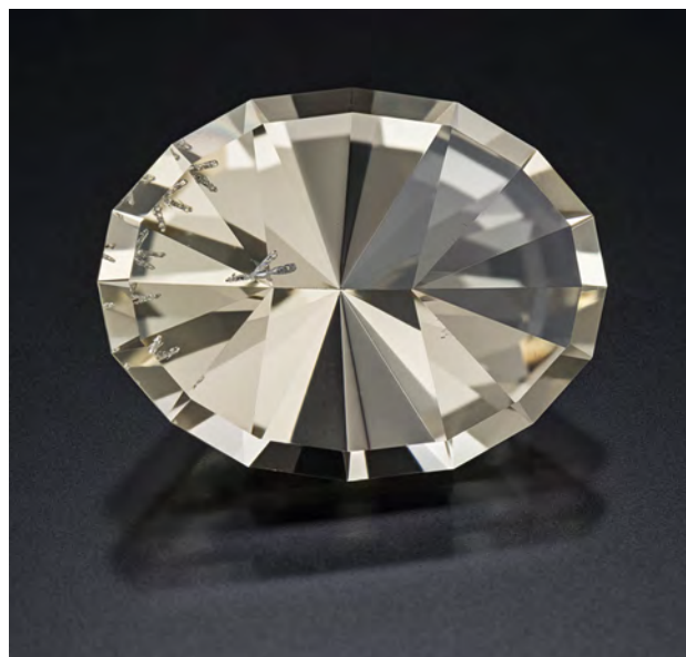
Figure 6. Located just left of center, a large apatite crystal cluster is visible directly below the table facet of this 7.20 ct orthoclase feldspar (the inclusion is also reflected numerous times by the pavilion facets). Photo by Kevin Schumacher.
