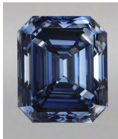
Figure 14. This 10.08 ct ( 13.54 \times 11.39 \times 7.36 mm) HPHT-grown diamond, with color equivalent to Fancy Deep blue, is the largest HPHT synthetic to date.
