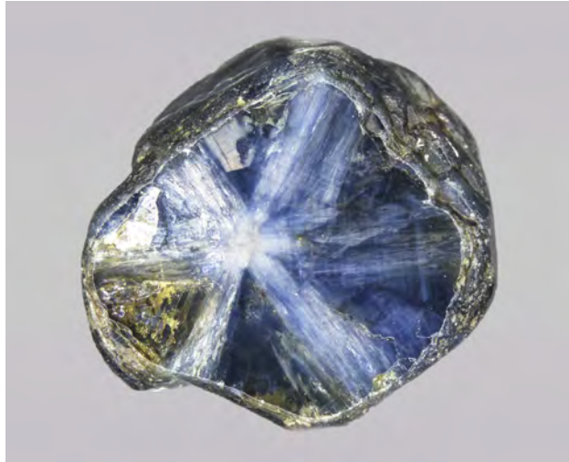
Figure 6. The polished section of the trapiche-type sample, as seen with fiber-optic illumination. The central white core and the six whitish particle-rich arms separated by blue areas are clearly visible. Photo by Victoria Raynaud.
