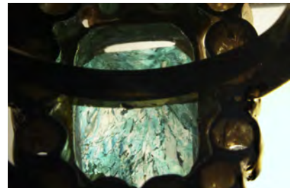
Figure 1. A green dye concentration in beryl was observed along fractures and confirmed by spectroscopic testing.
