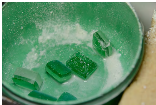
Figure 23. These triplets were assembled and preformed into rectangular shapes before being fashioned. Photos by Andrew Lucas, courtesy of Rhea Industries.
