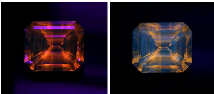
Figure 15. The blue synthetic diamond showed strong red-orange fluorescence to long-wave UV radiation (left) and yellow fluorescence to short-wave UV.
