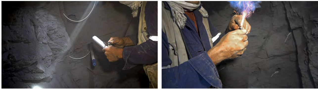
Figure 13. Hoping to reach an emerald-bearing pocket, the miners stuffed explosives into holes they had drilled and lit a fuse that subsequently lit all the fuses. Photos by Pedro Padua.
