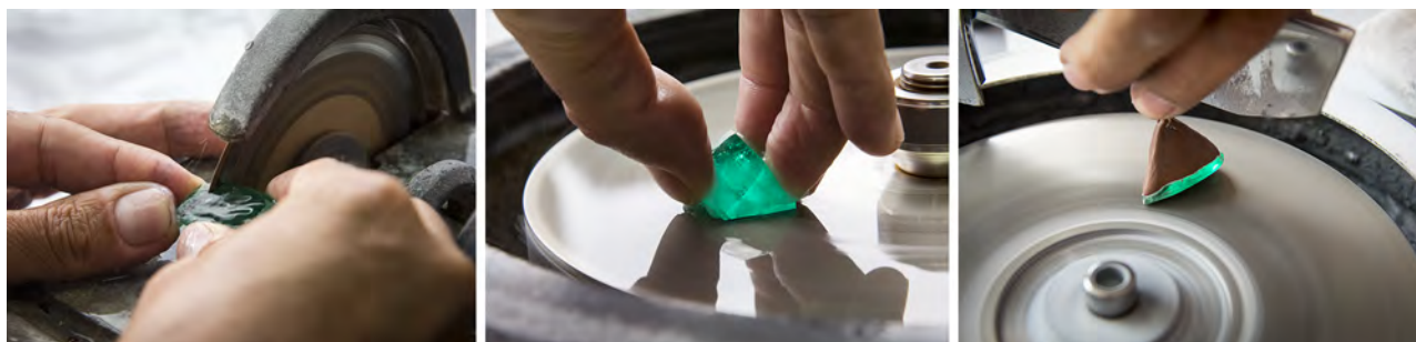
Figure 26. At The Best Emeralds , we followed the sawing and cutting of a 700 ct piece of rough and documented the decisions made from start to finish to achieve maximum weight and value. Photos by Andrew Lucas.
