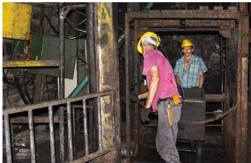
Figure 23. The La Pita operation uses elevators to bring up material from lower depths and carts to transport it through the tunnels. Photo by Andrew Lucas.
