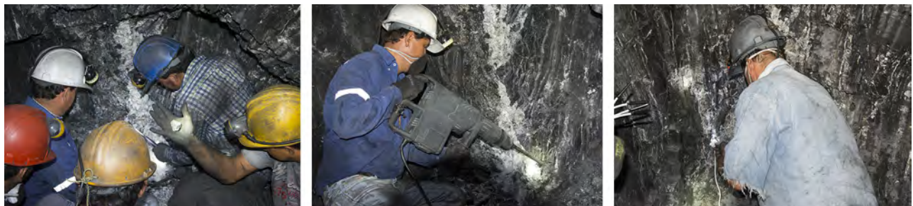
Figure 17. At Pavimentado, miners removed emerald-bearing pieces of calcite veins with hand tools and by drilling into the rock face, before placing explosives in the drill holes to advance the tunnel. Photos by Andrew Lucas.
