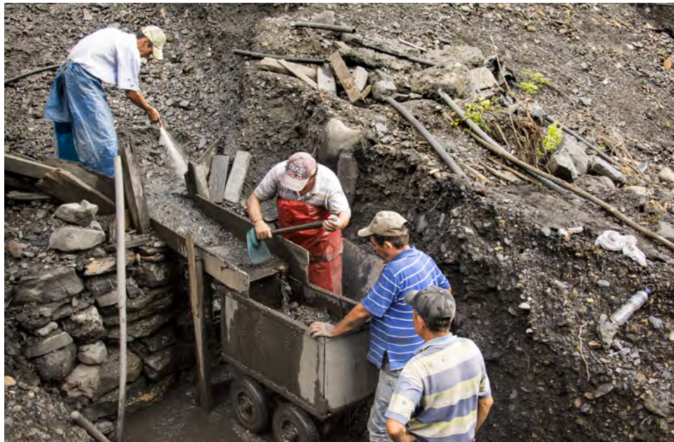
Figure 18. Independent miners on the banks of the Río Itoco use high-pressure water hoses to remove the shale, which will be washed in sluices or taken by wheelbarrow for washing. Photos by Andrew Lucas.
