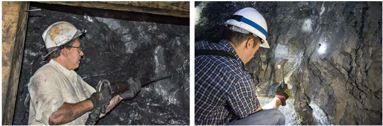
Figure 8. Two of the authors collected emerald directly from the deposits using hydraulic jackhammers to reach the emerald-bearing areas and then hand picks to remove the crystals from the host rock. Photos by Jonathan Muyal (left) and Andrew Lucas (right).
