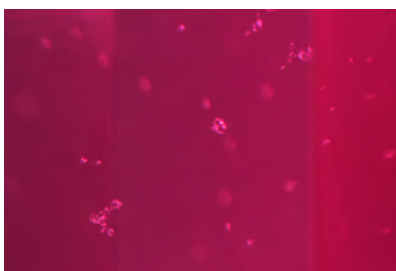
Figure 23. The abundance of transparent crystals and crystal clusters could easily be mistaken for a natural inclusion scene in a pink sapphire from Madagascar. Field of view 1.79 mm.
