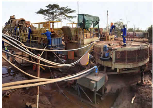
Figure 12. Mustang Resources’ new washing plant consists of two rotary pans equipped with trammel screens and log washers. Its current capacity is about 600 tons per day. Photo by Vincent Pardieu.
