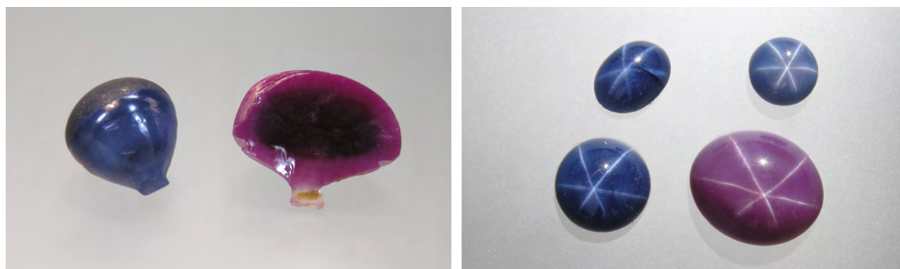
Figure 2. Synthetic asteriated corundum produced by Wiede's Carbidwerk. Left: Rough, almost spherical to elliptical boules of synthetic blue star sapphire and synthetic star ruby. The blue sapphire weighs 9.94 ct and measures 10.9 \times 10.0 mm; the ruby (one of the samples split at the center and shown from both sides in figure 3) weighs 11.57 ct and measures 14.8 \times 12.4 mm. Right: Three synthetic blue star sapphire cabochons and one synthetic star ruby cabochon in direct sunlight. The ruby weighs 8.92 ct and measures 13.2 \times 11.0 mm; the sapphire at the bottom left weighs 3.67 ct and measures 9.1 mm in diameter. Photos by K. Schmetzer.
