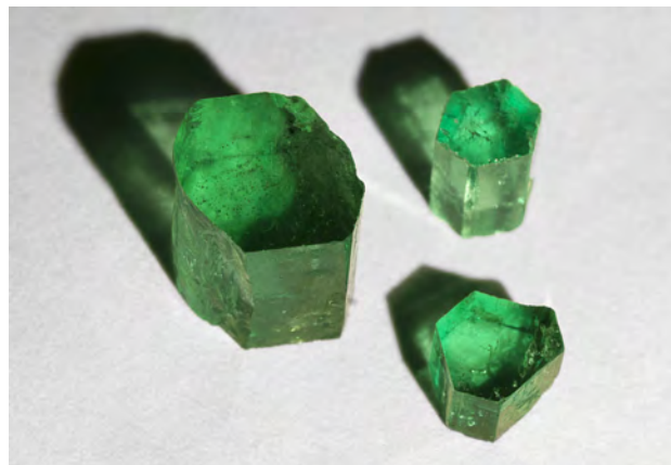
Figure 1. Emerald crystals from Colombia (top right), Afghanistan (bottom right), and Zambia (left). Each emerald's hexagonal prismatic crystal habit has been enhanced by polishing flat the two hexagonal end faces (perpendicular to the crystal's c-axis) and two or more prism sides (parallel to the c-axis). Photo by D.B. Thompson.
