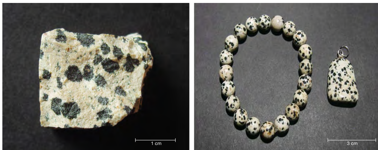
Figure 1. Dalmatian stone samples examined in this study reveal a spotted appearance connected with the presence of alkali amphiboles disseminated through feldspar-quartz matrices. Left: A rough block-shaped specimen measuring 1.5 \times 1.5 \times 1 cm. Right: A polished bracelet (1 cm bead diameter) alongside a pendant measuring 3 cm in length. Photos by Tomasz Powolny.
