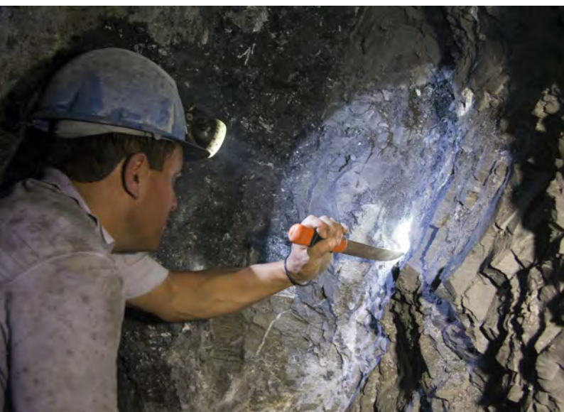
Figure 11. A variety of hand tools, including knives, were used at El Manantial to carefully remove emerald crystals from the productive zone. The tool chosen depended on how deeply the crystal was embedded in the rock and whether the miner felt it could be removed without damage. Photo by Andrew Lucas.
