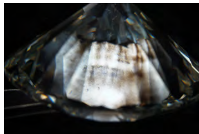
Figure 3. Tatami strain patterns, typical for a type Ia diamond, indicate that the crystal experienced plastic deformation during and possibly after growth.
