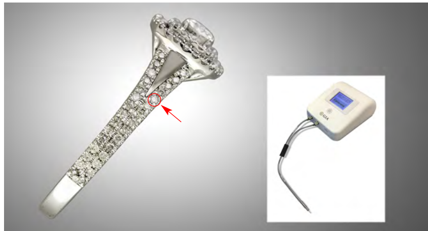
Figure 19. One stone, about 0.5 mm in diameter, was referred by the GIA iD100 for further testing. The inset photo shows a prototype of the iD100.
