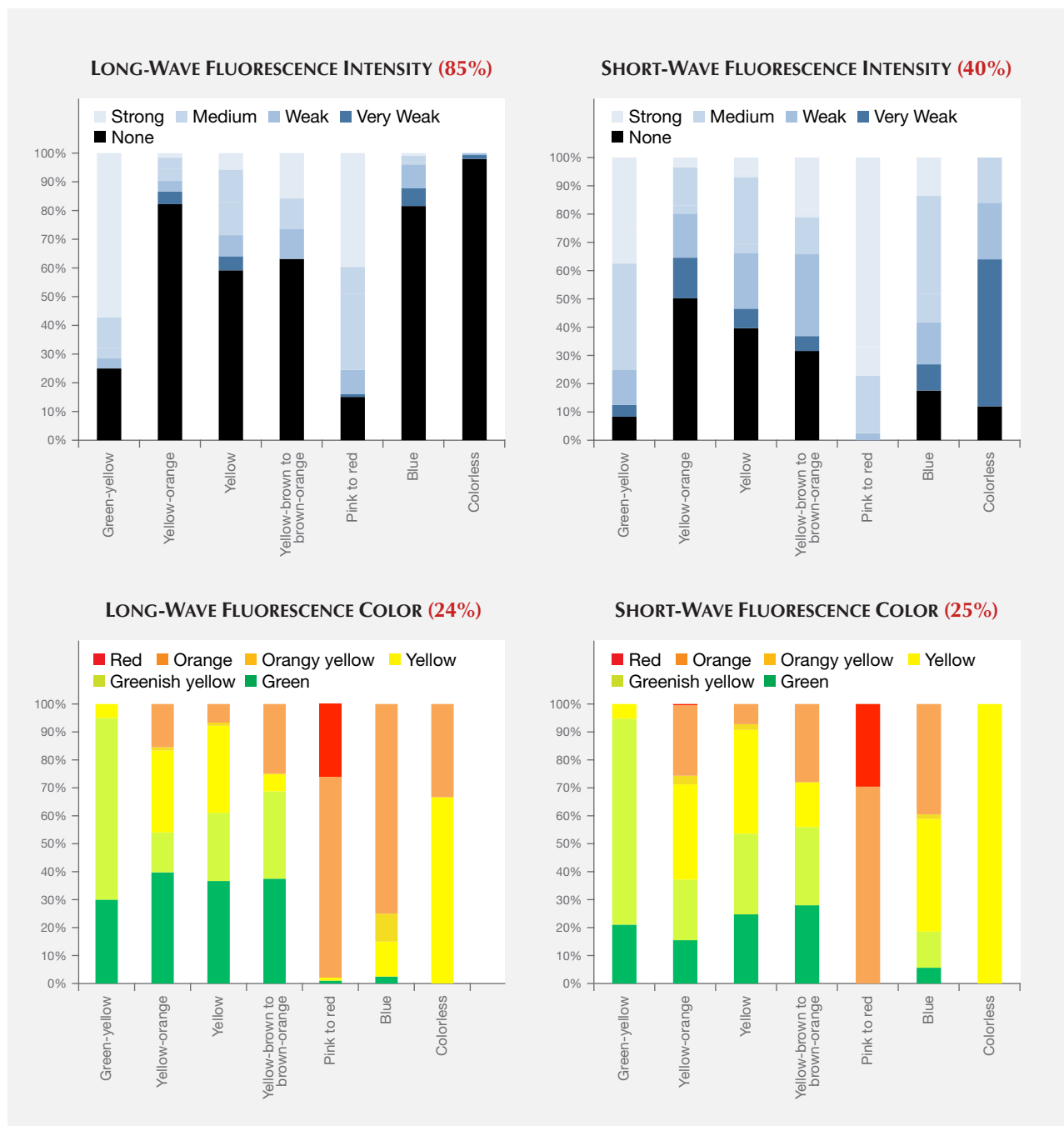
Figure 9. Fancy-color and colorless HPHT synthetics had distinctly different fluorescence reactions to long-wave and short-wave UV. Most of the HPHT synthetics showed no reaction to long-wave UV, while a majority showed an observable reaction to short-wave UV. The percentages shown in red represent the portion of samples for which data are available. The plots of fluorescence color only include those samples that had a reaction.
