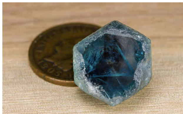
Figure 7. The rough sapphire after heating, with a window polished to view the interior. Photo by Jeffrey R. Hapeman.
