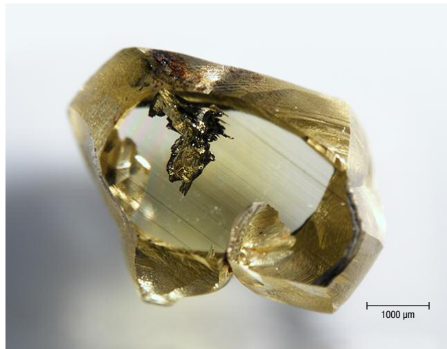
Figure 1. Left: Re-Os isotopic compositions for 10 sulfides from three Zimmi diamonds all fall along 650 Ma age arrays. Each diamond had multiple sulfides that lay on arrays of identical age, giving unequivocal evidence for the age and showing that these diamonds formed in the same episode of diamond formation. Right: Plane polarized light image of a typical sulfide inclusion in a polished Zimmi diamond plate. Note that this diamond only contains one inclusion, whereas analyses of three to four inclusions per diamond are shown in the plot on the left. From Smit et al. (2016), used with permission.
