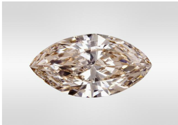
Figure 1. LPHT-treated brownish pink CVD synthetic diamond weighing 0.192 ct. Photo by Hiroshi Kitawaki.
