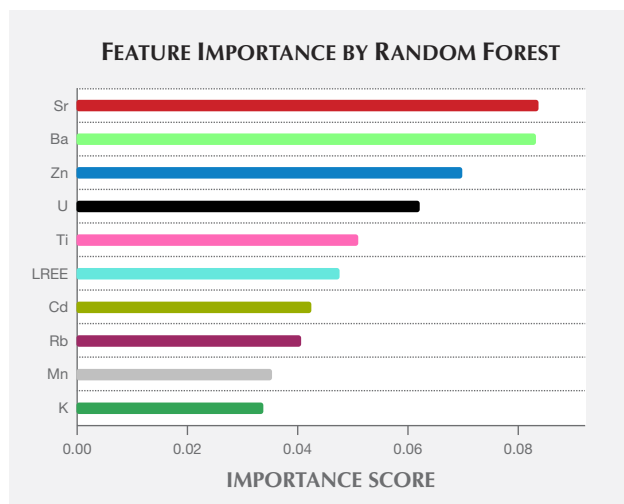
Figure 2. The 10 most important trace elements for green nephrite classification, ranked in descending order, analyzed by the random forest algorithm.
