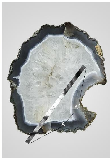
Figure 1. Left: The Borghese-Windsor Cabinet on display at the Getty Center, being imaged by the hyperspectral analyzer (center, on tripod). Right: This Brazilian agate from Rio Grande do Sul is part of the NHMLA collection. Transect A-A' is where the Raman map was collected. Photos by Arlen Heginbotham (left) and Aaron Celestian (right).
