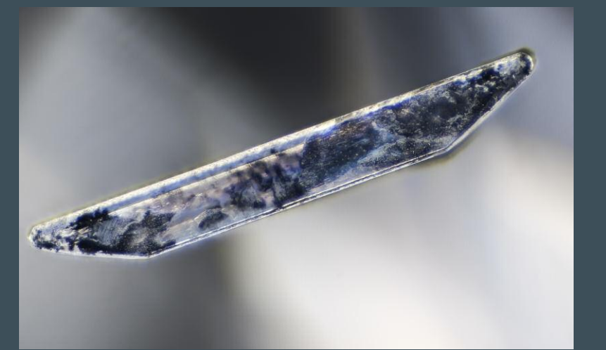
This flux-grown laboratory-grown diamond contains a large flux-filled negative crystal. Field of view 1.44 mm.
