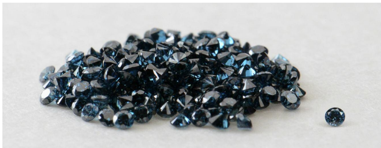
Figure 15. This group of 300 green-blue diamonds (1.97 carats total) was screened by GIA's Tokyo laboratory. Among these, 299 were irradiated natural melee diamonds and the one on the right was an irradiated CVD synthetic melee diamond.
