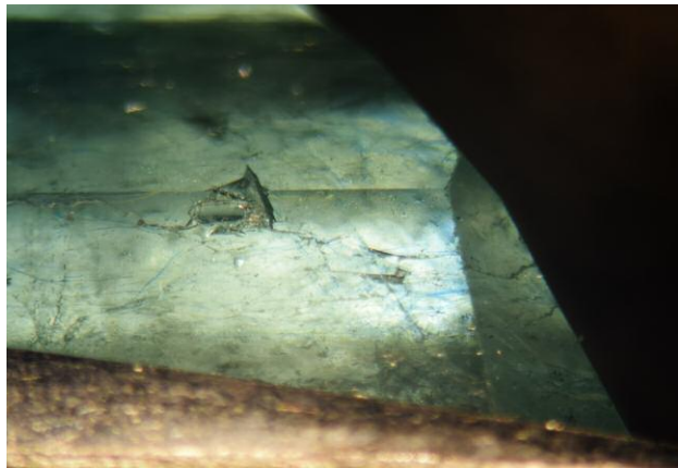
Figure 19. When viewed through a gemological microscope, “blue flashes” characteristic of resin-filled emeralds are clearly visible. Photo by Lai Tai-An Gem Lab; field of view 8.8 mm.
