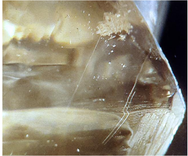
Figure 26. Needle-like inclusions in the rough synthetic moissanite sample. Photo by V. Pakhomova.
