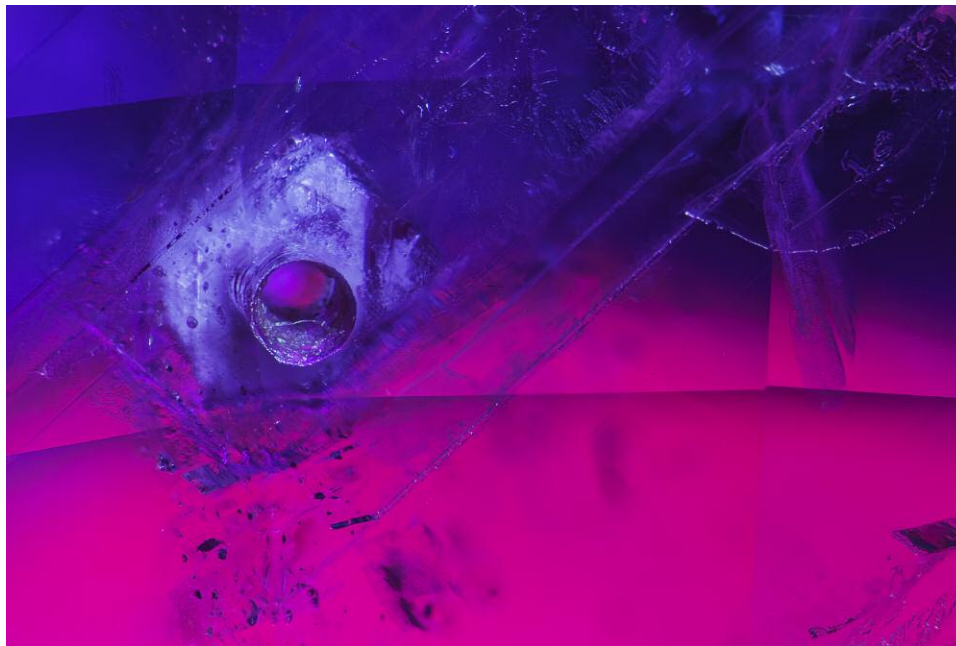
Figure 4. A drill hole in a heated pink sapphire from Myanmar, seen with diffuse brightfield and fiber-optic illumination. Photomicrograph by E. Billie Hughes; approximate field of view 5 mm.
