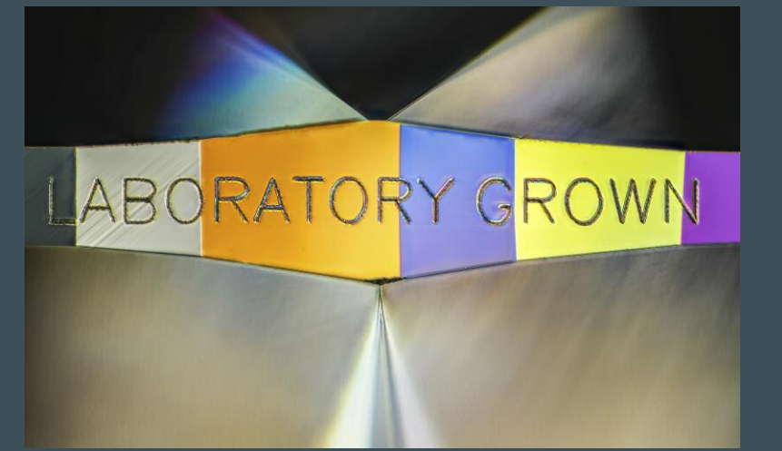
The girdle may contain information showing that a diamond is man-made, as seen here using differential interference contrast. Field of view 1.44 mm.
