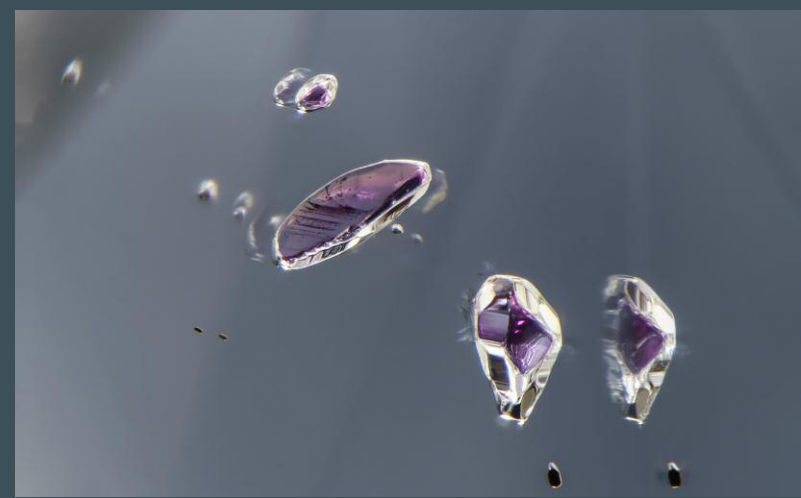
Bright purplish pink chromian garnets are a relatively common type of colored inclusion in gem diamonds and indicate peridotitic origin. Field of view 1.99 mm.
