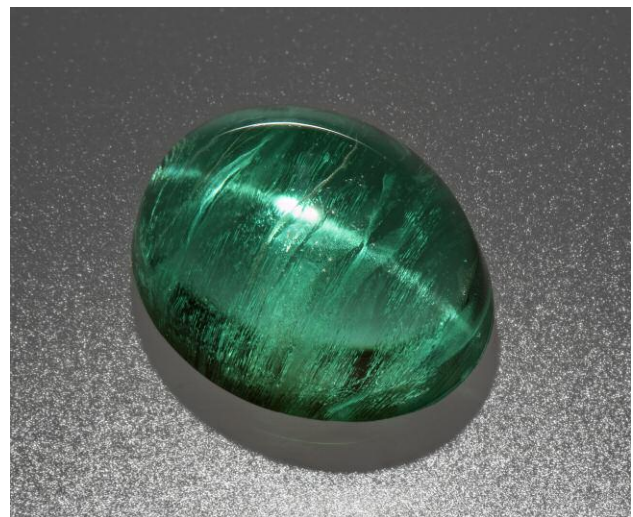
Figure 6. This 2.73 ct Gilson synthetic emerald cabochon displays a sharp "cat's-eye" phenomenon. Photo by Kevin Schumacher.
