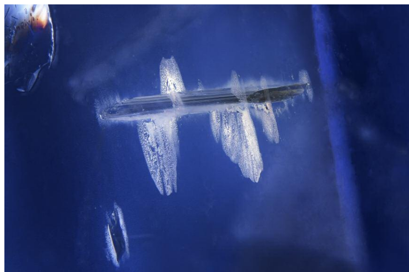
Figure 13. A large prismatic pargasite mineral inclusion. Field of view 7.19 mm.
