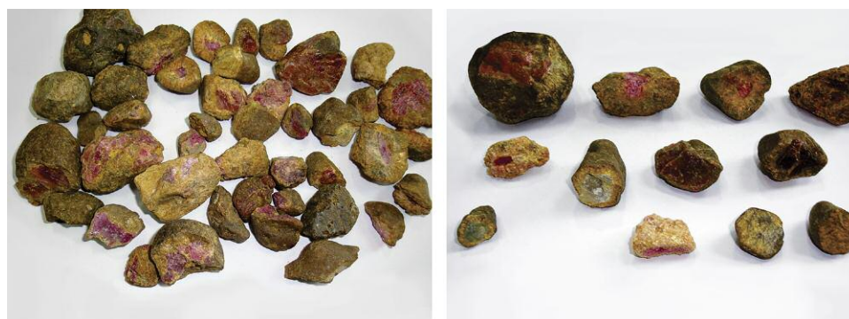
Figure 6. Left: Rough stones from the Truc Lau secondary deposit, some of which contain a spinel corona. Right: Twelve pieces of corundum with spinel corona were selected from the lot and used for this study. Photos by N.N. Khoi.
