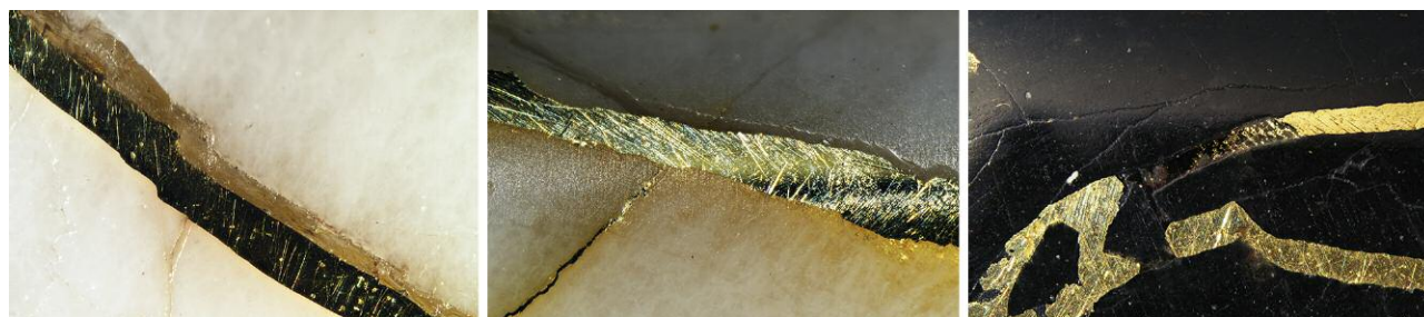
Figure 6. Unnatural veins in manufactured gold-in-quartz. Left: This vein is filled with both polymer, which is not flush with the host quartz, and gold (field of view 4.79 mm). Center: A vein of polymer running alongside a vein of gold with undercutting visible at the boundary of the polymer vein and the host quartz (field of view 3.57 mm). Right: Polymer fills an incomplete gold vein; the rest of the vein is recessed below the host quartz (field of view 7.19 mm).
