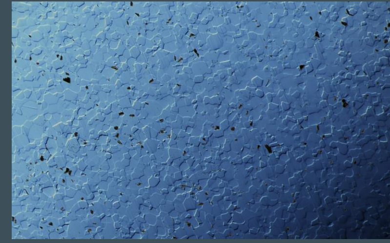
Interlocking grains with different crystallographic orientations show undercutting in this polycrystalline diamond. Field of view 2.88 mm.
