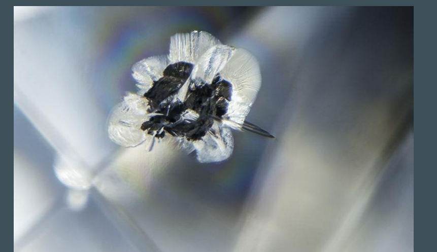
Black carbon inclusions that stand out in high relief are occasionally seen in CVD-grown diamonds. Field of view 1.42 mm.
