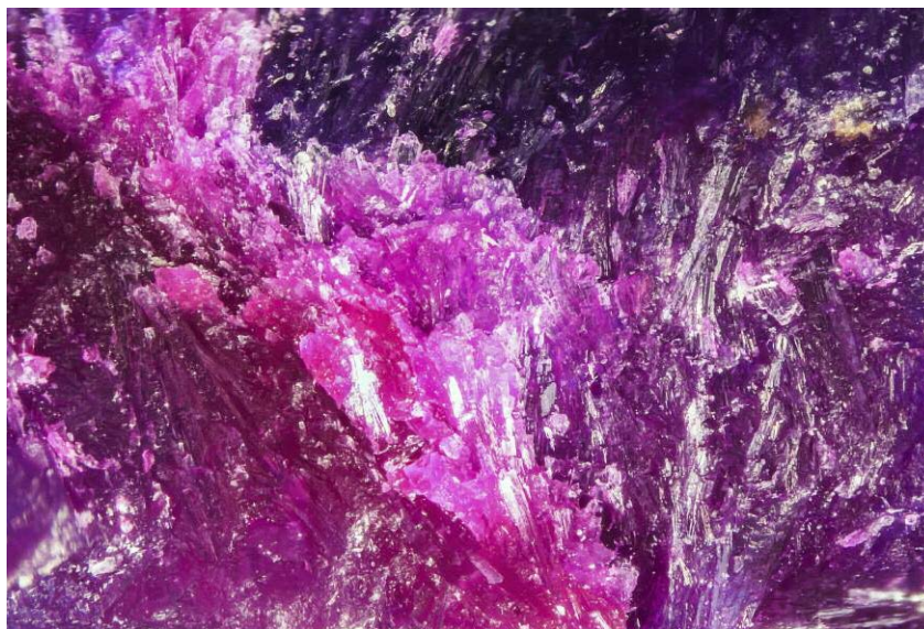
Figure 16. The fibrous internal structure of the specimen resembling sugilite was actually consistent with serpentine. Field of view 4.11 mm.
