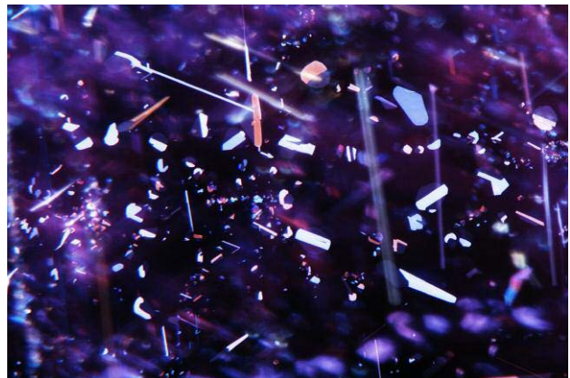
Figure 12. Reflective particles and platelets are very common but take some practice to observe with a fiber-optic light. Photo by B. Kongsomart; field of view 1.35 mm. Fiber-optic illumination.
