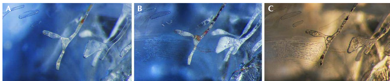
Figure 10. A: Before heating, sample 10 is filled with elongated negative crystals, some of which branch into “Y” shapes. Many of these are filled with orange stains, but most are removed after acid cleaning. B: After the first round of heat, to 800°C, some changes are already apparent. The orange staining has turned a darker brownish shade. Some of the negative crystals, like the one on the right, have started to display a “frosty” white appearance on the surface. In the background behind the negative crystals, we can see faint signs of fissures and fingerprints beginning to develop. C: When heated to 1000°C, the changes become more pronounced. Some of the tubes, like the one in the center, have developed immobile bubbles inside. The fissures from previous rounds of heating have also begun to heal and create clear fingerprints composed of small channels. Also note how the background color has changed from medium blue to near-colorless. Diffuse oblique fiber-optic illumination. Photomicrographs by E. Billie Hughes; field of view 1 mm.
