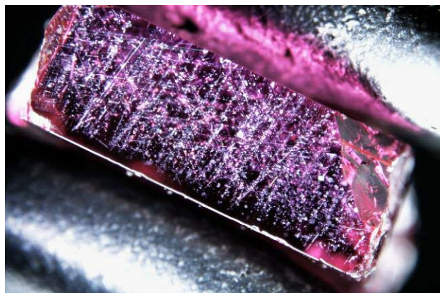
Figure 14. The ruby from figure 13 shows a variety of particles and platelets when a fiber-optic light is shined through it at the correct angle. Photo by GIA; field of view 12.3 mm.
