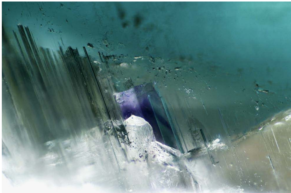
Figure 3. A Russian emerald hosts a crystal inclusion—identified by laser Raman microspectrometry analysis as fluorite—that exhibits a distinct purple color. Photomicrograph by Jonathan Muyal; field of view 1.44 mm.
