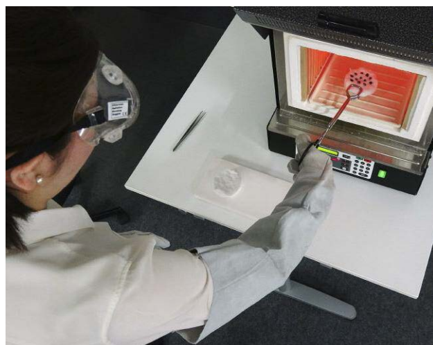
Figure 4. E. Billie Hughes removes the samples from the Vulcan 3-550 oven after a heating session. Photo by Rosey Perkins.
