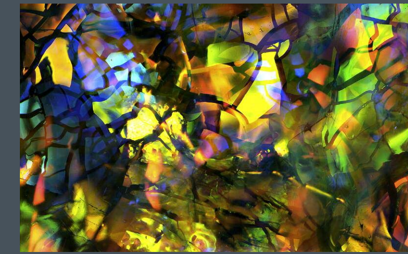
Slocum Stone opal imitation glass was manufactured by John Slocum of Michigan in the early 1970s. Thin layers of metallic film fragments suspended in the glass matrix are responsible for the interference colors observed. Field of view 5.75 mm.
