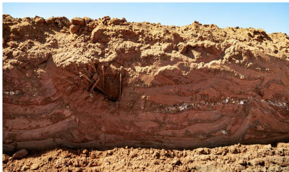
Figure 5. At the Mugloto pit, operated by MRM, a gravel layer containing rubies and quartz boulders in the secondary deposits is clearly visible. A tunnel that was supported by wooden structures is an indication that artisanal miners used to work in this area. Photo by Wim Verriest.
