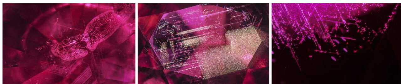
Figure 18. Inclusion scenes in Montana rubies. Left: A decrepitation halo surrounding an inclusion. Field of view 2.23 mm. Center: Angular bands composed of loosely to densely packed particles and short to long needles. Field of view 3.57 mm. Right: Oriented needles and platelets. Field of view 1.26 mm. Photomicrographs by Aaron Palke (left and right) and Tyler Smith (center).
