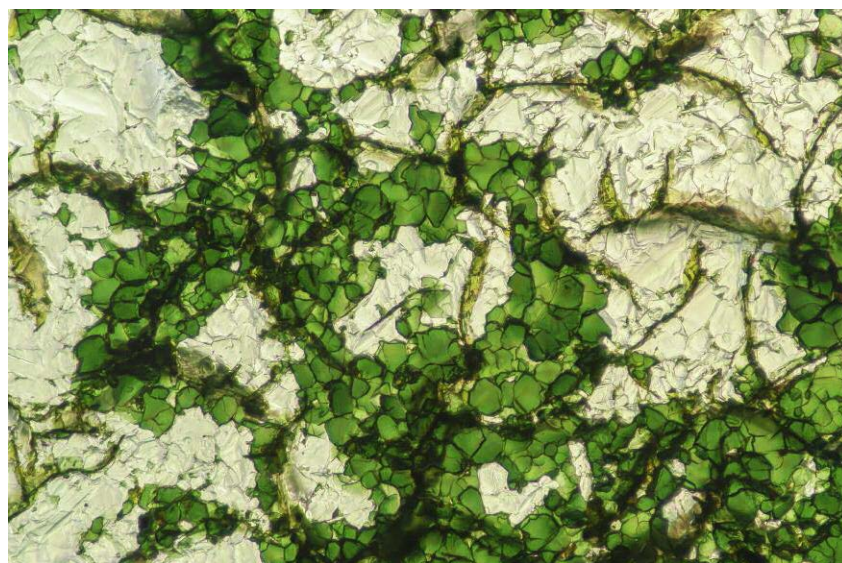
Figure 5. The diamond's patchy green coloration is caused by interlocking platy crystals of chromium oxide, visible with magnification. Field of view 0.72 mm.
