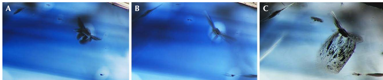
Figure 7. A: In sample 4 before heating, a cluster of transparent crystals surrounded by winged stress fractures has decolorized areas around them. B: After the first round of heating at 800°C, we can already observe small changes, as two of the crystals have developed larger glassy fractures than they had originally. C: By the time the sample is heated to 1100°C, significant differences have emerged. The previously smooth and glassy fissures around the crystals have become larger and begun to heal, creating a “fingerprint” appearance. Also note that the decolorized areas are much less prominent, and that the overall blue color of the stone has become lighter. Brightfield illumination, with blue and white diffusing filters. A blue diffusing filter is used to color-correct the light source, which has a yellow tint, to make it more neutral. Photomicrographs by E. Billie Hughes; field of view 1.8 mm.
