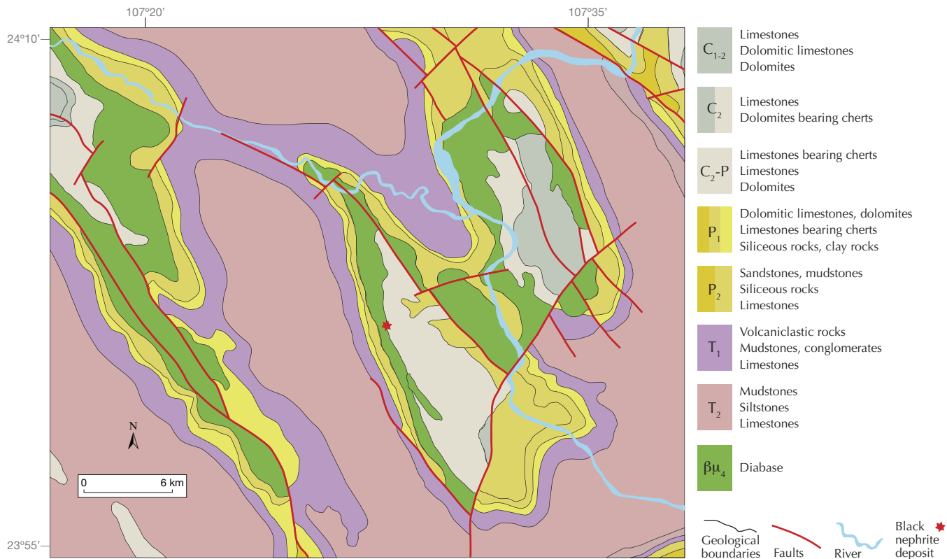
Figure 3. Regional geologic map of the Guangxi black nephrite primary deposit. The deposit occurs at the contact zone between marine carbonate rock bearing chert/siliceous rock/clay rock deposited from the Upper Carboniferous to Lower Permian periods (C 2 -P 1 ) and diabase emplaced during the late Permian period (βμ 4 ). The diabase displays an obvious circular structure in anticlines extending northwest to southeast and is controlled or transformed by several faults extending northwest by north, northeast by north, and northeast by east (modified after the 1:200000 geologic map from the National Geological Archives of China).
