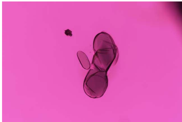
Figure 16. These two greenish amphibole crystals, identified by Raman spectroscopy, represent the most common crystal inclusion in Mozambican ruby. The smallest shows the typical rounded, elongated shape, while the larger crystal has a more irregular shape. Photo by C. Khowpong; field of view 1.42 mm. Brightfield illumination.
