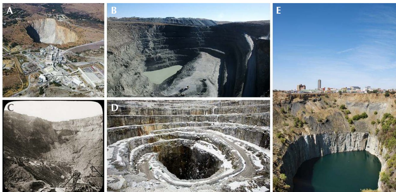
Figure 1. Open-pit diamond mines in kimberlite rock. Mining operations remove as much kimberlite as possible and leave deep pits that outline the shape of a “kimberlite pipe.” A: The Cullinan mine started as an open-pit operation and transitioned to underground mining in 1946. Photo by DeAgostini/Getty Images. B: Active mining in one of the kimberlite pipes at the Letšeng mine. Photo by Karen Smit/GIA. C: The Kimberley mine “Big Hole,” where mining was completed in 1914. Photo by The Print Collector/Getty Images. D: The bottom of the open pit in the Diavik mine. Photo by Ben Nelms/Bloomberg via Getty Images. E: The “Big Hole” of the Kimberley mine today. Photo by Karen Smit/GIA.
