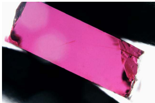
Figure 13. A Mozambican ruby appears clean when viewed in brightfield illumination. Photo by GIA; field of view 12.3 mm.
