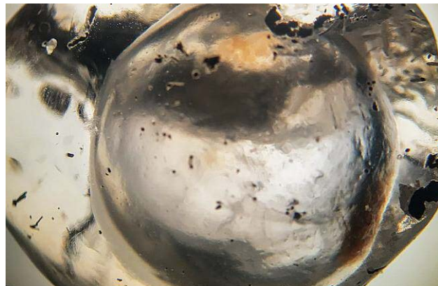
Figure 6. This eye-visible three-phase fluid inclusion in a Mexican opal was just over 14 mm in diameter and contained solid, liquid, and gaseous phases. Photomicrograph by Nathan Renfro.
