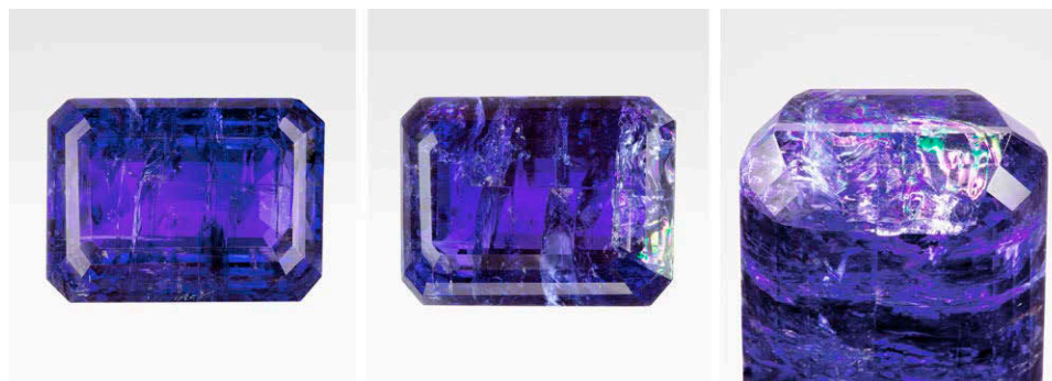
Figure 18. This large 115 ct tanzanite was found to contain oil (left). After removal of the oil (center and right), highly reflective fissures became obvious. This clearly demonstrates how oiling a gem can have a radical impact on its appearance. Photos by Chanon Yimkeativong.
