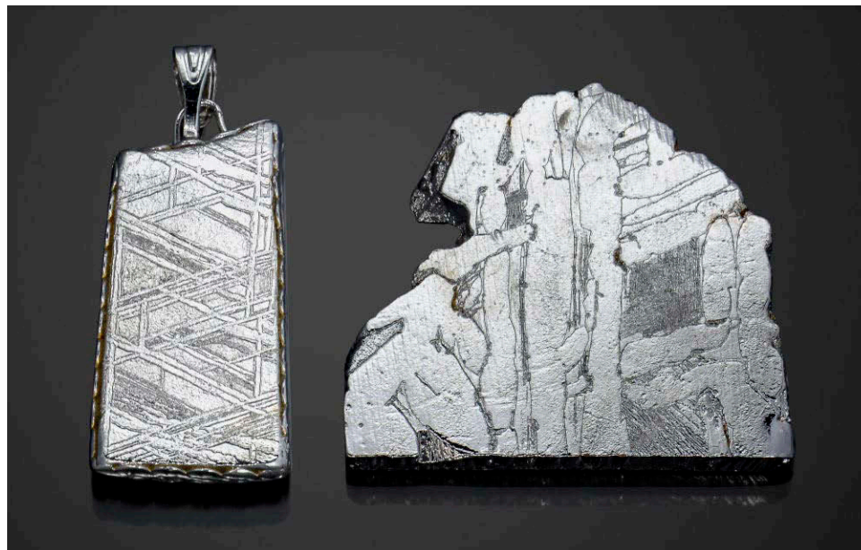
Figure 16. The meteorite pendant (left) measured 27.02 × 12.75 × 2.59 mm and weighed 28.53 ct. The meteorite slab (right) measured 27.67 × 28.06 × 1.71 mm and weighed 36.69 ct. The intricate banding seen in these plated meteorites would both be categorized as Widmanstätten patterns, features of octahedrite iron meteorites. Photo by Angelica Sanchez.
