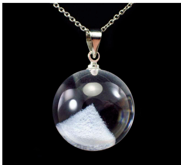
Figure 12. The “phantom quartz” pendant was later confirmed to be natural quartz with three-dimensional laser engraving. Photo by Shu-Hong Lin.
