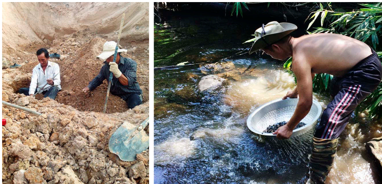
Figure 3. Left: Artisanal miners use crowbars and shovels to remove topsoil and dig through the gem-bearing layer in the Binh Thuan gem field. Right: Gem-bearing gravels are washed and sieved along the stream at Dak Nong. Photos by Doan Thi Anh Vu.
