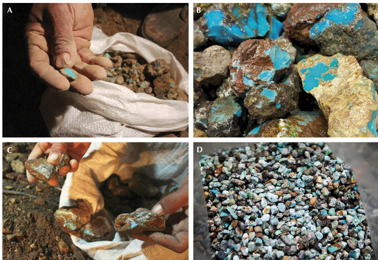
Figure 25. The four major quality levels of rough turquoise production from Neyshabur: turquoise nuggets (A), turquoise with the host rock attached (B), chalky turquoise (C), and turquoise chips (D). Photos by B. Shirdam.
