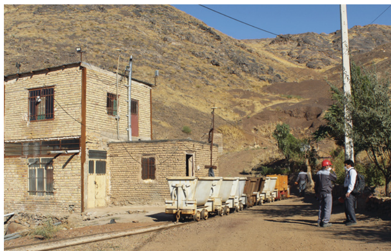
Figure 24. At the Dom tunnel's entrance, the wagons are returned to the mine after emptying the waste. Photo by B. Shirdam.
