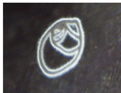
Figure 18. Micro image of the largest spiral marking; the line thickness is 40 microns.
