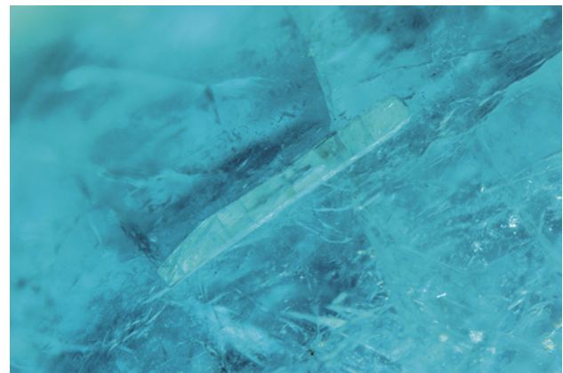
Figure 11. A tourmaline inclusion in Brazilian Paraíba tourmaline. Photomicrograph by Suwasan Wongchacree; field of view 4.8 mm.
