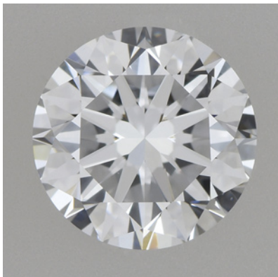
Figure 1. Face-up view of the 1.497 ct, E-color HPHT-processed diamond submitted in 2021 for update service.
