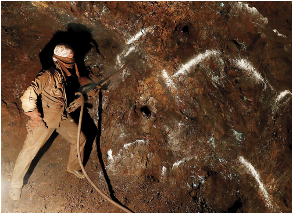
Figure 21. A drilling crew prepares to dig a blast hole. Photo by M. Bakhshandeh Zahmati.
