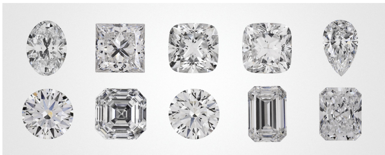
Figure 13. These 10 CVD-grown diamonds submitted to the New York laboratory were fairly large (2.24 ct to 5.90 ct) with high color grades (D to F) and excellent clarity (VVS 2 to VS 1 ).
