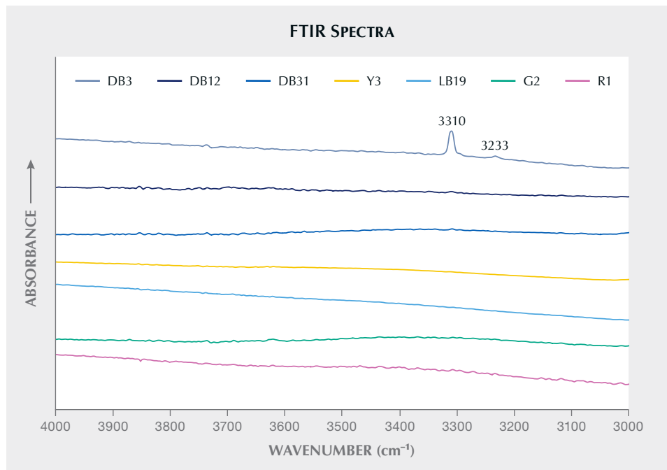
Figure 19. The FTIR spectra of representative samples from each group. Samples DB3, DB12, and DB31 were selected to represent the deep blue group, in which DB3 displayed sharp peaks at 3310 and 3233 \text{cm}^{-1} . Samples Y3, LB19, G2, and R1 represented other groups with no significant peaks shown in the 4000–3000 \text{cm}^{-1} range. Spectra are offset vertically for clarity.
