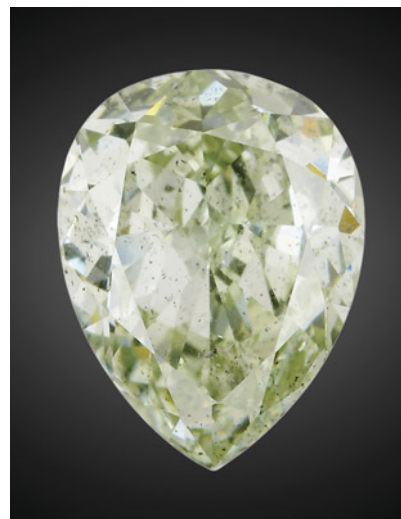
Figure 2. This 2.12 ct Fancy yellow-green diamond owes its color to both the nickel-related absorption band and the artificially introduced GR1 absorption.
