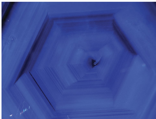
Figure 16. Well-defined hexagonal color zones in this deep blue stone indicate the crystallization process of the host sapphire. Photomicrograph by Yimiao Liu; field of view 3.94 mm.
