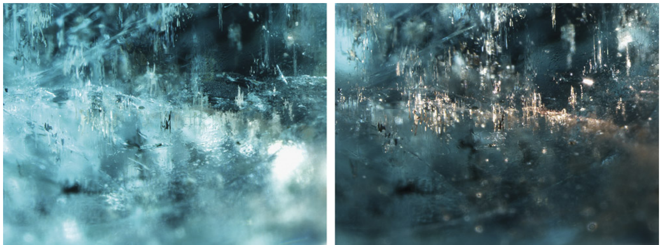
Figure 24. The copper inclusions aligned in the same direction appear brownish and black (left) and together display golden luster when the light enters from a certain direction (right). Field of view 2.3 mm.
