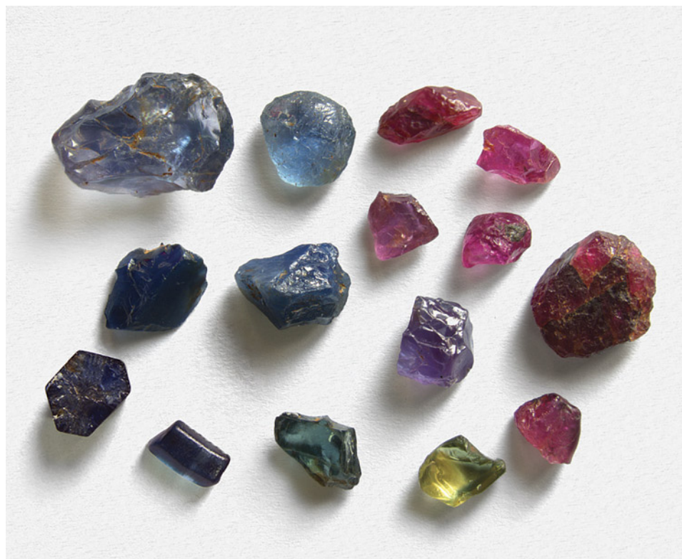
Figure 7. Rough stones from Muling, representing the five color groups from this study: two light blue sapphires (top left), four deep blue sapphires (bottom left), seven from the red group (including pink and purple samples; right), one green sample (bottom center), and one yellow sample (bottom right). The deep blue sapphires displayed well-developed barrel or tabular crystal shapes and predominantly hexagonal prisms. The light blue sapphires showed rounded shapes and erosion surfaces, while the red group consisted mainly of broken pieces with erosion surfaces or tabular crystals. The green and yellow samples were all broken pieces. Photo by Yimiao Liu.
