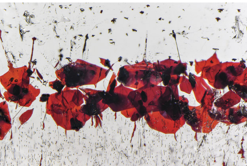
Figure 3. Red hematite crystals in quartz. Photomicrograph by Nathan Renfro; field of view 7.22 mm.
