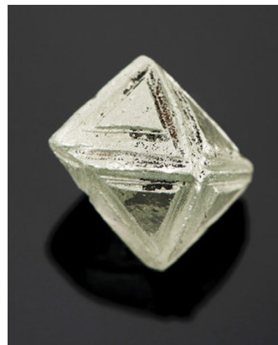
Figure 18. This 7.42 ct light bluish green synthetic moissanite, submitted as a diamond, displays triangular features on each of the octahedral faces.
