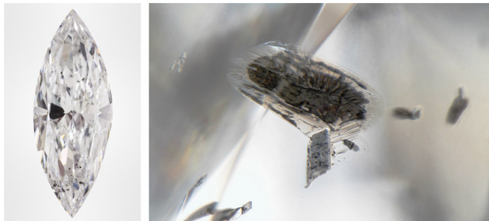
Figure 2. Left: A type IIa diamond (4.12 ct, D color) with metallic inclusions. Photo by Jian Xin (Jae) Liao. Right: The large metallic inclusion has a localized round, graphitized fracture extending from its top end. Photomicrograph by Evan M. Smith; field of view 1.42 mm.
