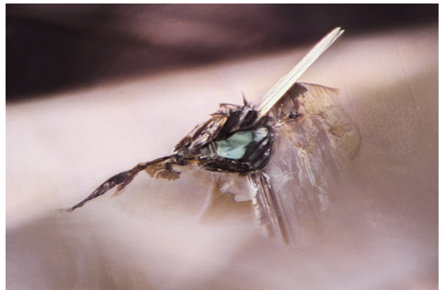
Figure 7. A bluish green omphacite crystal with surrounding stress fractures seen in a Fancy brown-pink diamond. Photomicrograph by Britni LeCroy; field of view 1.42 mm.
