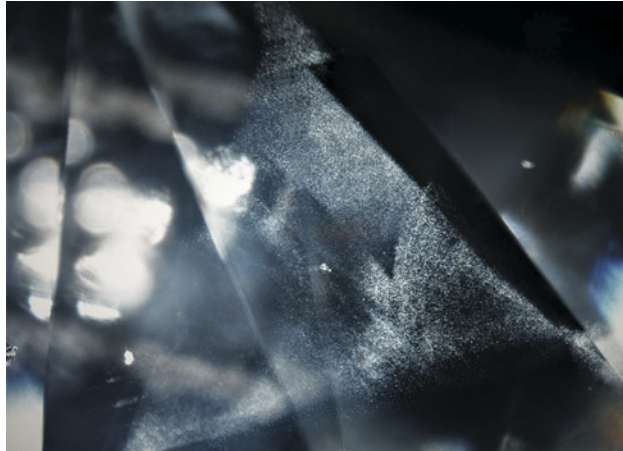
Figure 5. This particle cloud, a typical inclusion in diamond, shows an iridescent appearance and is grouped in a triangular shape viewed in fiber-optic illumination. Photomicrograph by Aprisara Semapongpan; field of view 2.8 mm.
