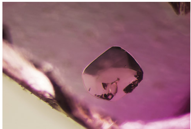
Figure 8. Spinel crystals, such as this one in sample 15, were seen frequently in the Burmese ruby samples. Photomicrograph by E. Billie Hughes; field of view 3 mm.
