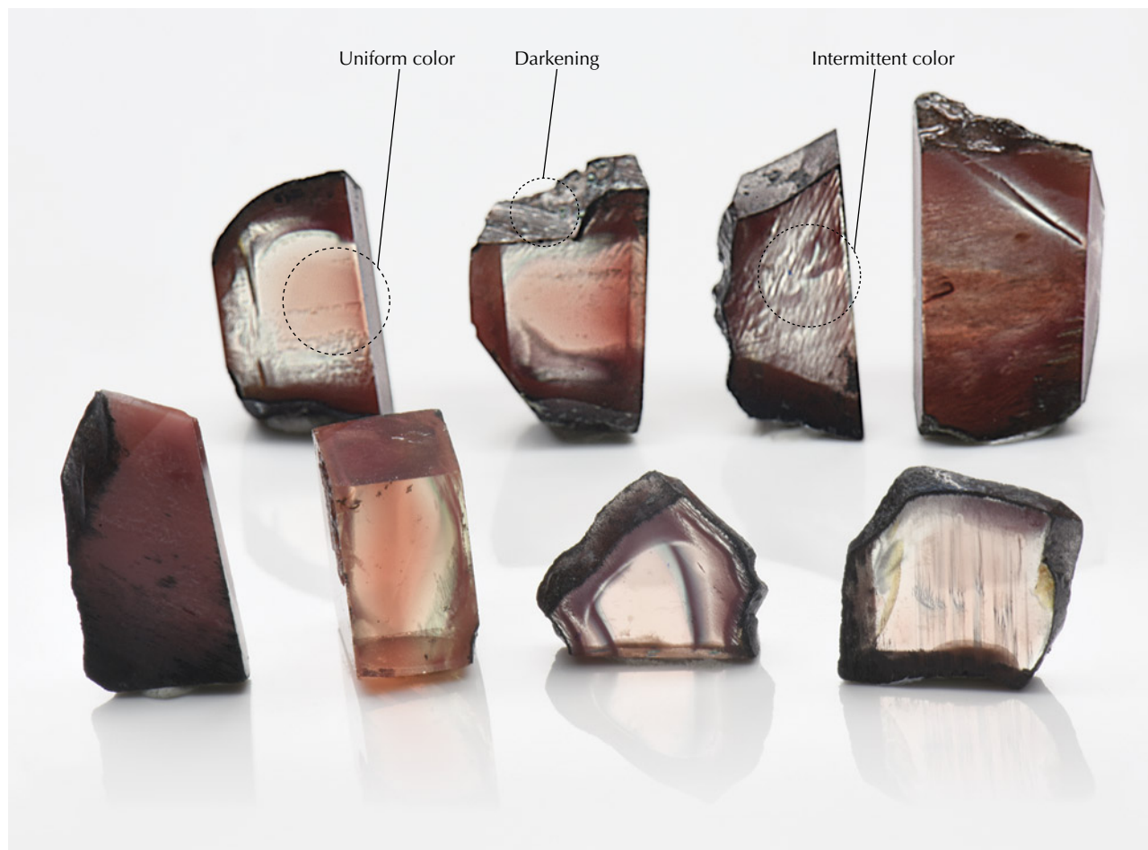
Figure 3. The copper-diffused labradorite feldspar samples used in this study (1.73–4.15 ct). Note that the surfaces were repolished after copper diffusion treatment. Photo by Chengsi Wang.
