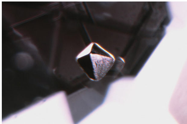
Figure 8. An octahedral fluorite crystal in a 1.25 ct Brazilian alexandrite. Photomicrograph by Hikaru Sato; field of view 2.37 mm.
