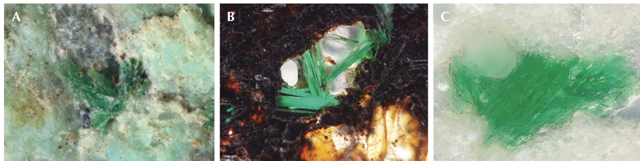
Figure 13. A: Bright green atacamite crystals associated with turquoise. B: Elongate columnar atacamite in matrix. C: Irregularly granular atacamite surrounded by quartz in matrix. Photomicrographs by Ling Liu; fields of view 1.1 mm (A) and 0.6 mm (B and C).
