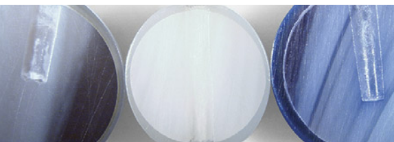
Figure 25. Left to right: Cross sections of an irradiated akoya pearl, a white akoya pearl, and an irradiated and dyed akoya pearl. Field of view 14.52 mm.
