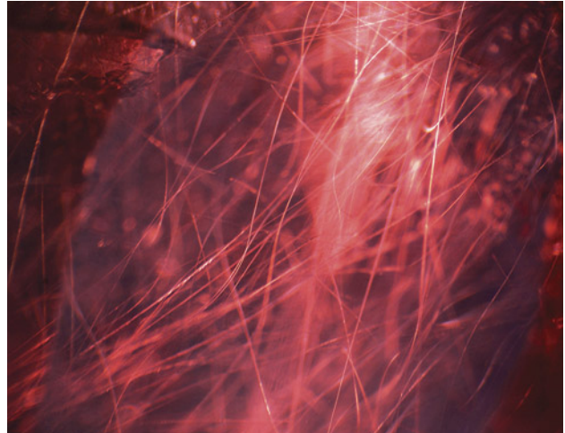
Figure 18. Many long tube inclusions were observed in the rhodonite sample. Photomicrograph by Chunyan Wang; field of view 2.36 mm.
