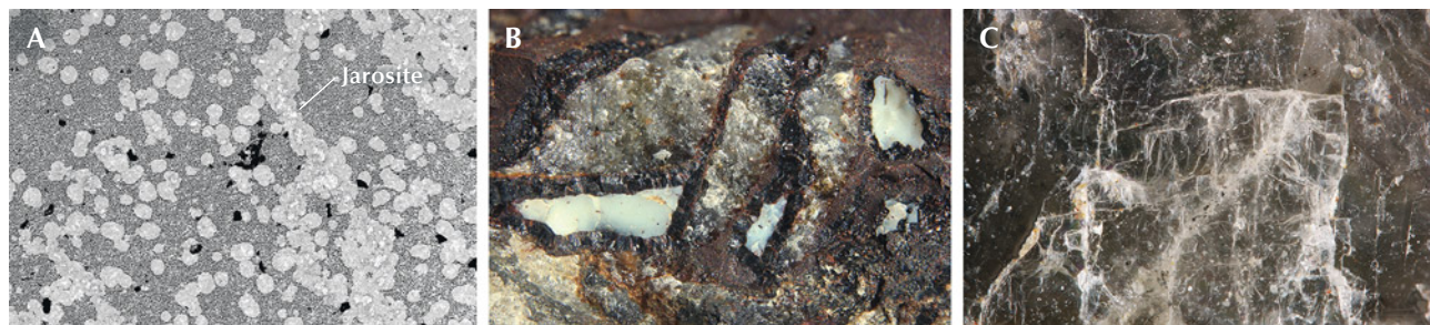
Figure 17. A: Jarosite has the brightest gray value in this BSE image. B: Bonattite with a milky appearance filling in the fissures and wedge-shaped cavities of goethite. C: Muscovite with perfect cleavage, found in the matrix of rough samples. Photomicrographs by Ling Liu; fields of view 1.2 mm (A), 5.9 mm (B), and 1.1 mm (C).
