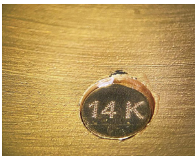
Figure 11. The hallmark is not actually stamped onto the metal but is on a separate disk adhered to the inside of the bracelet.
