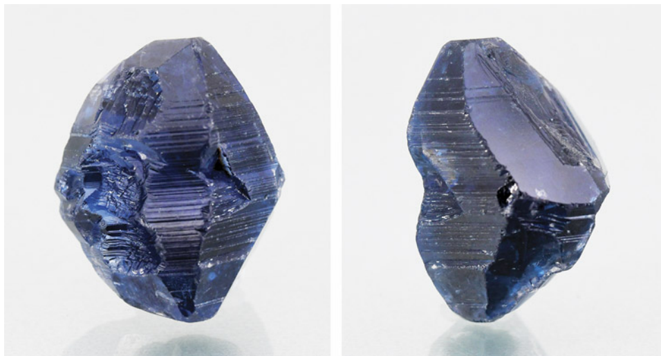
Figure 18. This unusually large 64.70 ct rough specimen displaying a bipyramidal crystal habit and stepped striations was identified as a flux-grown synthetic sapphire. Note the large rhombohedral face in the image on right. Photos by Gagan Choudhary.
