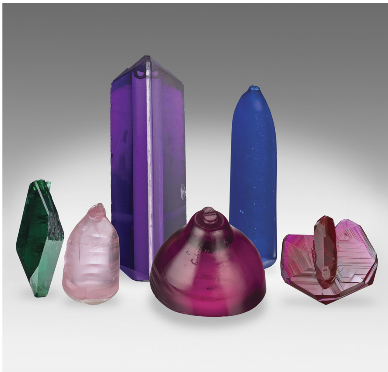
Figure 16. Synthetic crystals from the GIA Museum collection. Left to right: Russian hydrothermal synthetic emerald, flame-fusion pink synthetic spinel, hydrothermal synthetic amethyst with a colorless seed plate, titanium-doped Czochralski-grown purplish pink synthetic sapphire boule, flame-fusion blue synthetic spinel boule, and flux-grown Ramaura synthetic ruby. Photos by Robert Weldon.
