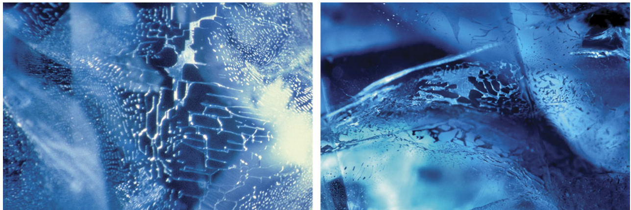
Figure 8. Images showing the similarity between fingerprints in some natural sapphires (left) and flux-healed fingerprints in some flux-grown synthetic sapphires (right), which could lead to confusion between the two. Photomicrographs by John I. Koivula.
