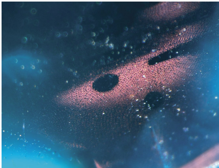
Figure 29. Further magnification revealed the arrangement of particles in a moiré pattern. Field of view 0.93 mm.
