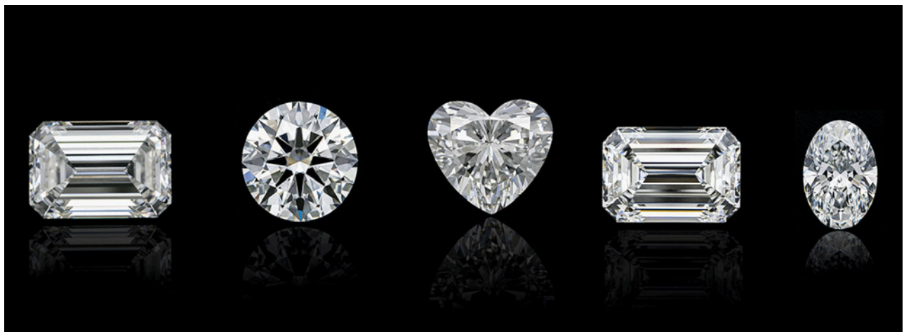
Figure 18. Large laboratory-grown diamonds such as these CVD-grown diamonds have become increasingly common the last few years. From left: a 12.06 ct G-color, VS 2 emerald cut; an 11.36 ct E-color, SI 1 round brilliant; a 10.42 ct G-color, VS 2 heart brilliant; a 10.19 ct F-color, VS 2 emerald cut; and a 9.52 ct E-color, VS 2 oval brilliant. Photos by Gaurav Bera.
