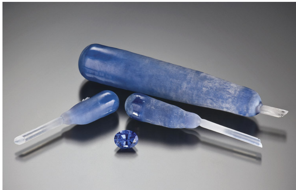
Figure 4. Flame-fusion synthetic sapphire boules and an oval-cut gem (2.45 ct). Photo by Robert Weldon. Cut stone gift of Aaland Gem Co. Inc., GIA Museum no. 24224.
