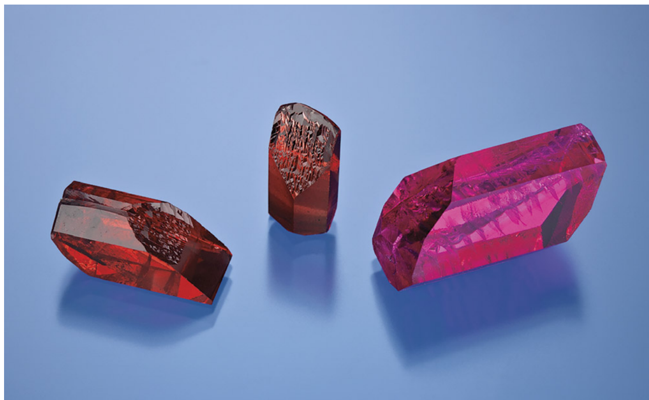
Figure 14. Hydrothermally grown synthetic beryl ranging from 1.08 to 6.32 g. Photo by Robert Weldon.
