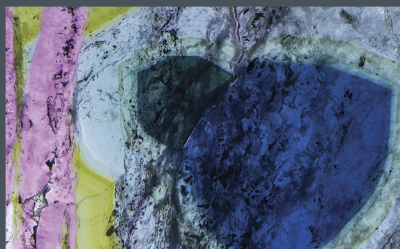
A slice of elbaite tourmaline from Brazil shows complex color zoning when viewed perpendicular to the c-axis of the crystal. Field of view 13.43 mm.
