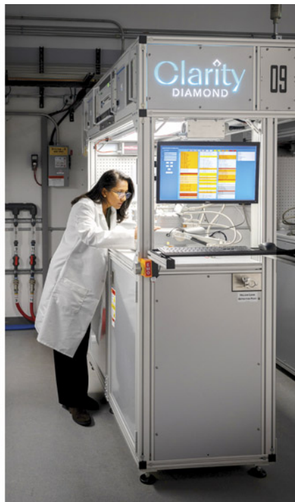
Figure 14. A CVD-grown diamond factory such as Clarity's facility in Austin often has rows of reactors lined up (left). The reactors are carefully monitored throughout the growth period, as demonstrated by process engineer Dr. Amanda Charris (right). Courtesy of Clarity Diamond.
