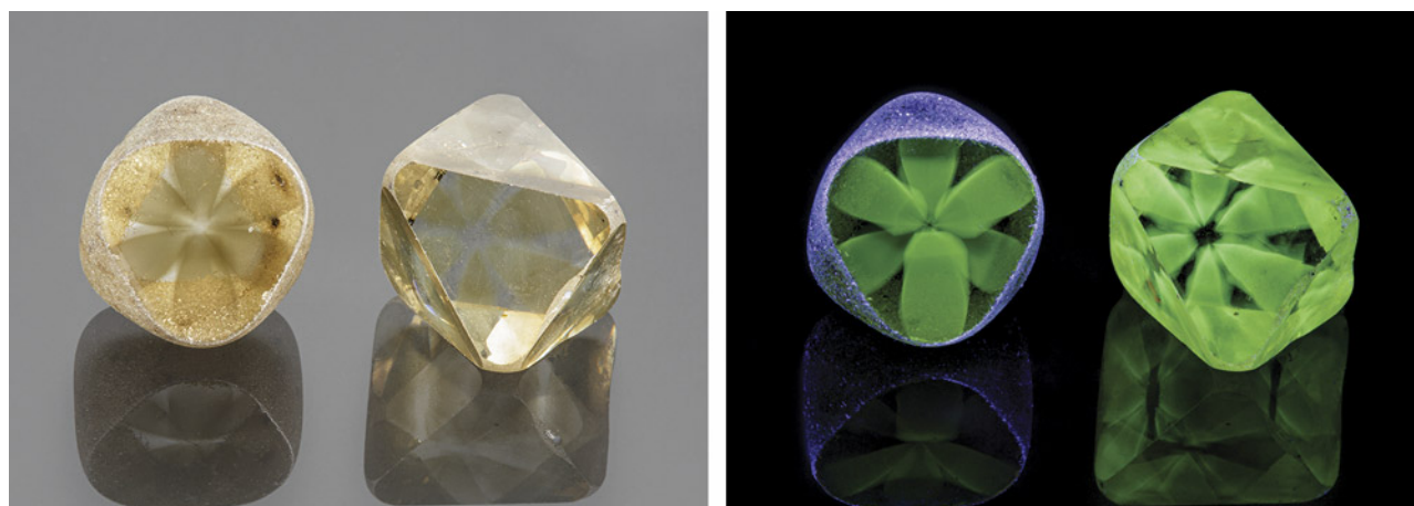
Figure 3. Left: An 8.14 ct and an 8.57 ct diamond containing brown asteriated cloud inclusions with sixfold symmetry. Right: The clouds fluoresced green when exposed to long-wave UV. The purple reflections of the UV source are likely caused by surface imperfections on the rough surface.
