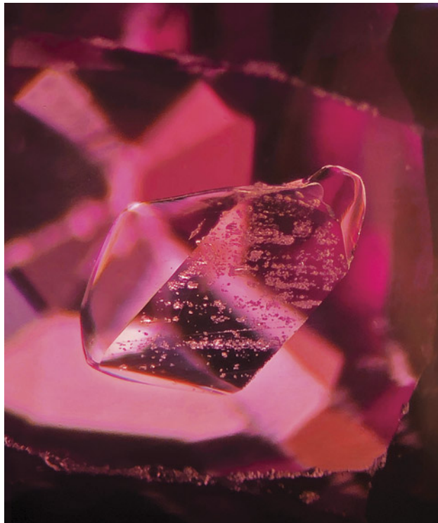
Figure 16. A large surface-reaching spinel inclusion in a Burmese pink sapphire from Mogok, shown in dark-field and oblique illumination. Photomicrograph by Kyaw Thu; field of view 1.3 mm.
