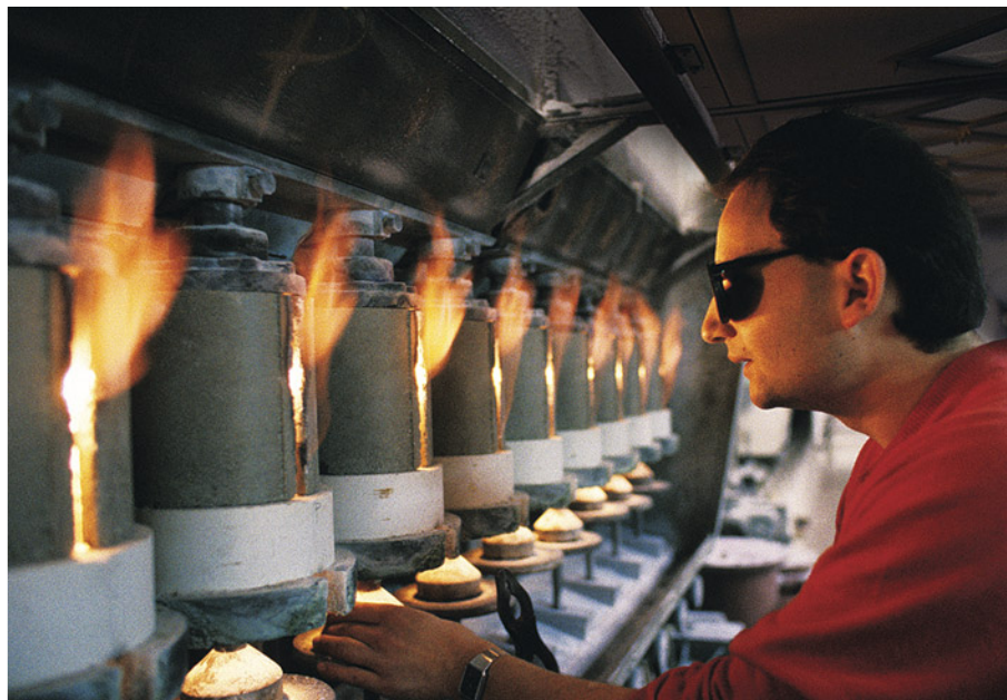
Figure 3. Drawing of a Verneuil (flame-fusion) apparatus (left) and a photo of flame-fusion crystal growth in the furnace (right). Photo courtesy of Hrand Djvahirdjian.
