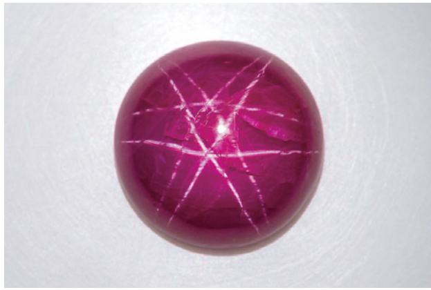
Figure 12. This unheated 11.43 ct purplish red round ruby cabochon displayed a white twelve-rayed double-star phenomenon. Photo by Nuttapol Kitdee.
