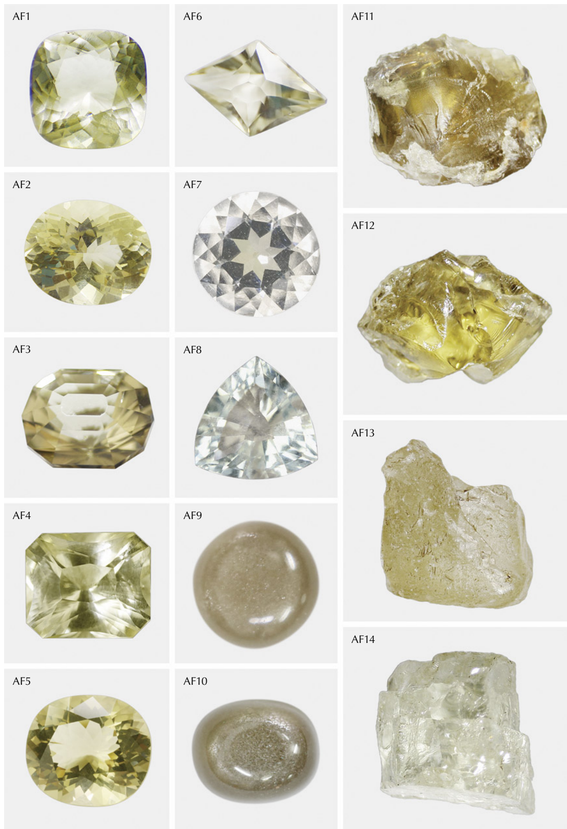
Figure 4. Anorthoclase samples from this study consisted of eight faceted stones, two cabochons, and four rough samples within three color groups: near-colorless, brownish gray, and yellow. Photos by Le Ngoc Nang.
