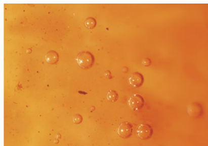
Figure 13. Microscopic observation of the 89.81 ct sphere revealed unnatural color patches (left) and gas bubbles and trapped dirt (right). Fields of view 19.20 and 1.80 mm.
