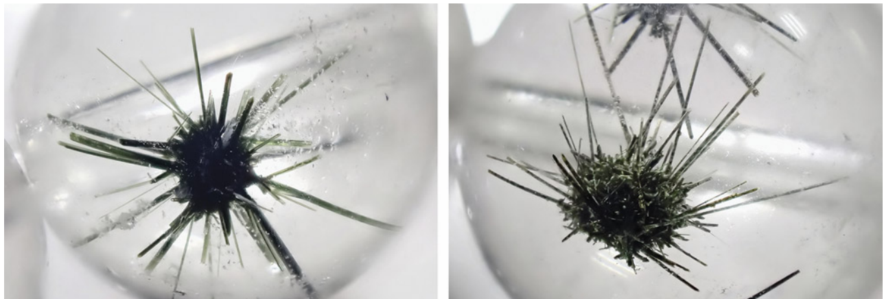
Figure 12. These dark green acicular aggregates in quartz were identified as hedenbergite. Photomicrographs by Liyan He; fields of view 9.20 mm (left) and 8.30 mm (right).
