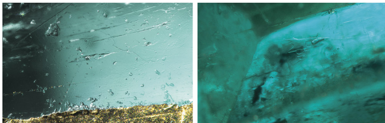
Figure 5. Inclusions in two emeralds from the pendant shown in figure 2. The jagged three-phase inclusions support a Colombian origin. Photomicrographs by Aaron Palke; fields of view 1.76 mm (left) and 1.99 mm (right).
