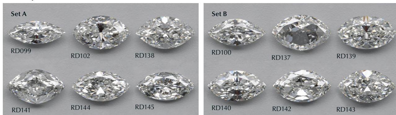
Figure 3. These virtual images display the 36 research diamonds used for observations, grouped into sets A and B for each shape. They range in size from 0.33 to 0.86 ct, have color grades between D and K, and have clarities between VVS_2 and I_1 . Table 1 contains size and grading-report information for each diamond. The images were created with a proprietary rendering configuration, mimicking the DiamondDock environment. Still virtual images and videos of these stones in motion are available online ( https://www.gia.edu/gems-gemology/fall-2024-fancy-shaped-diamonds ).
