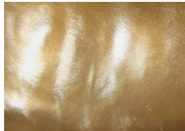
Figure 21. A linear-looking nacre is characteristic of nacreous Pinna or pen pearls from the Pinnidae family; field of view 3.68 mm.
