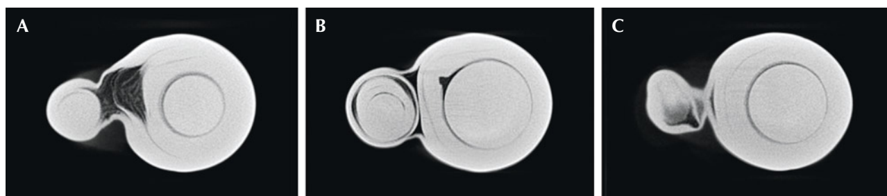
Figure 26. \mu -CT scan images of the saltwater bead cultured pearl at different depths.
