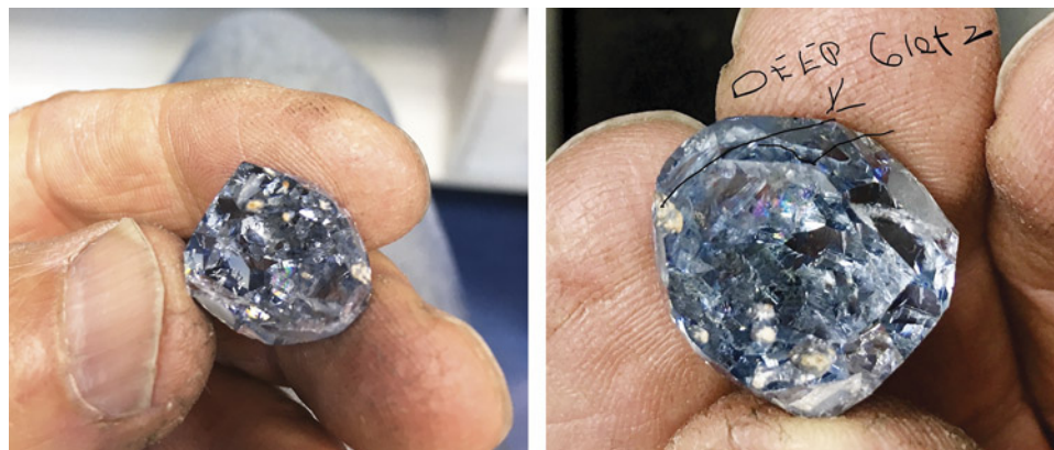
Figure 34. Lieberman examines a 40 ct rough blue diamond that yielded a 15 ct heart. The lines on the right photo indicate where the stone might be sawn. Photos courtesy of Harvey Lieberman.
