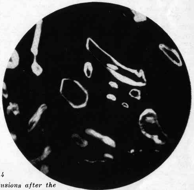
Fig. 3 Group of phantoms and irregular in- clusions containing carbonic acid in a light blue aquamarine at normal room temperature. 100x.
