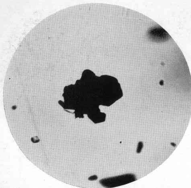
Figure 7 Yellow sapphire from Ceylon, containing group of distinctly outlined tabular hematite crystals. Included crystals of other minerals are never present in synthetics. Gemological microscope.
