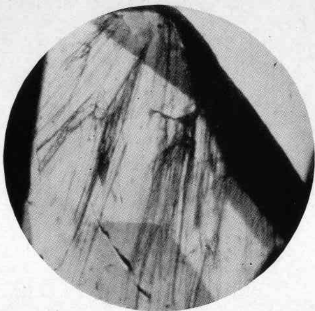
Figure 3 Byssolite threads as inclusions in demantoid. 50x.
