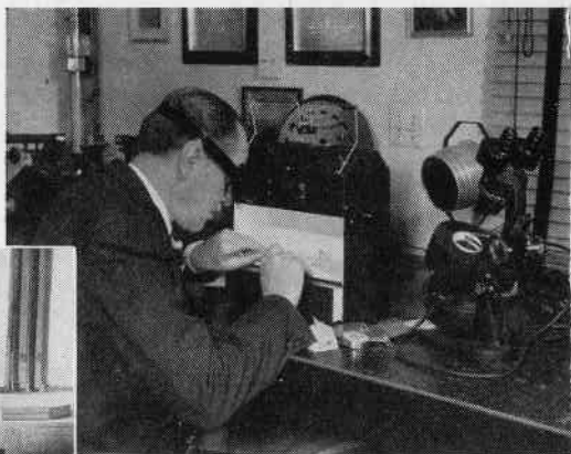
The Diamondscope at the left and at the top the Diamondlite with yardstick for color grading of diamonds in the GIA Laboratory. At the bottom of the page is shown the X-ray Diffraction Unit.
