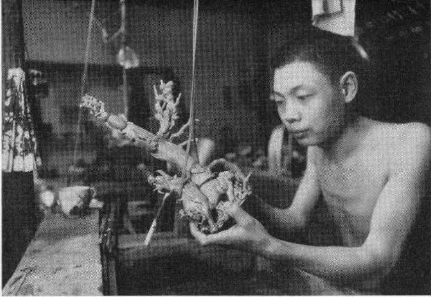
Finishing an elaborate pink coral goddess mounted on a Chinese unicorn or "Ch'i-lin." At the left are a number of spindles with assorted cutting heads.
