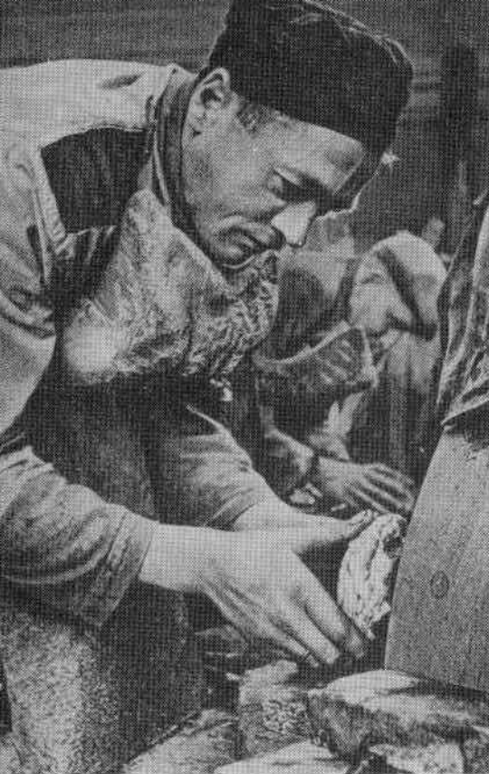
The rotating beech-tree trunk smeared with tripoli powder for polishing stones is now but occasionally employed.
