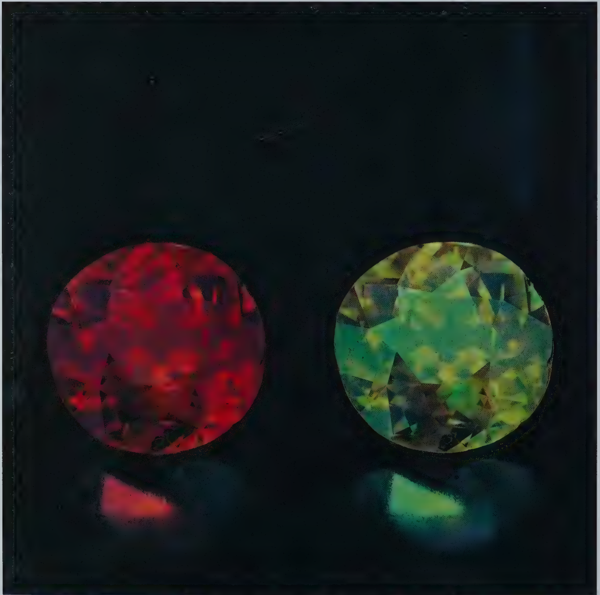
An 8.9-ct. alexandrite from Sri Lanka, showing its color change—in incandescent light (red) and in daylight (green).
