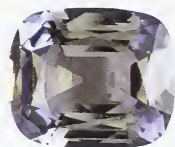
SILLIMANITE 111 Distinctly pleochroic, good cleavage
