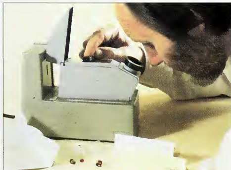
SEEING DOUBLE Zircon's back facets look doubled, due to strong double refraction (DR).
