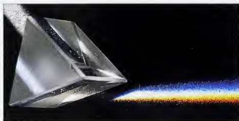
SPLITTING LIGHT THROUGH A PRISM The splitting of white light into its spectral colors is called dispersion. It gives gems their internal fire.
