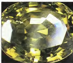
SEEING DOUBLE Zircon's back facets look doubled, due to strong double refraction (DR).
