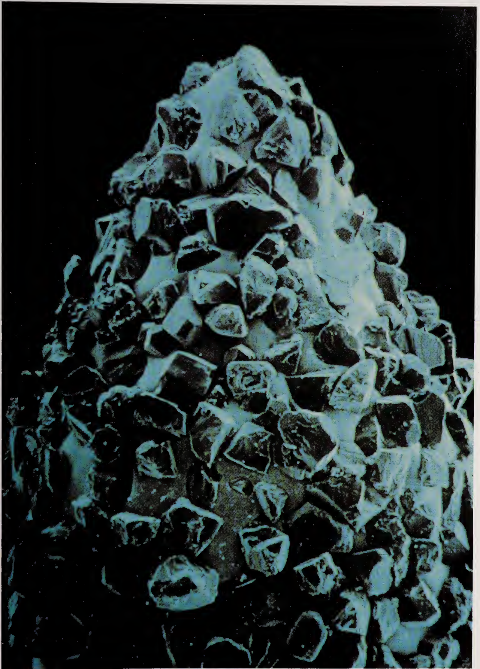
An electron microscope photograph of the diamond chips on a dental drill
