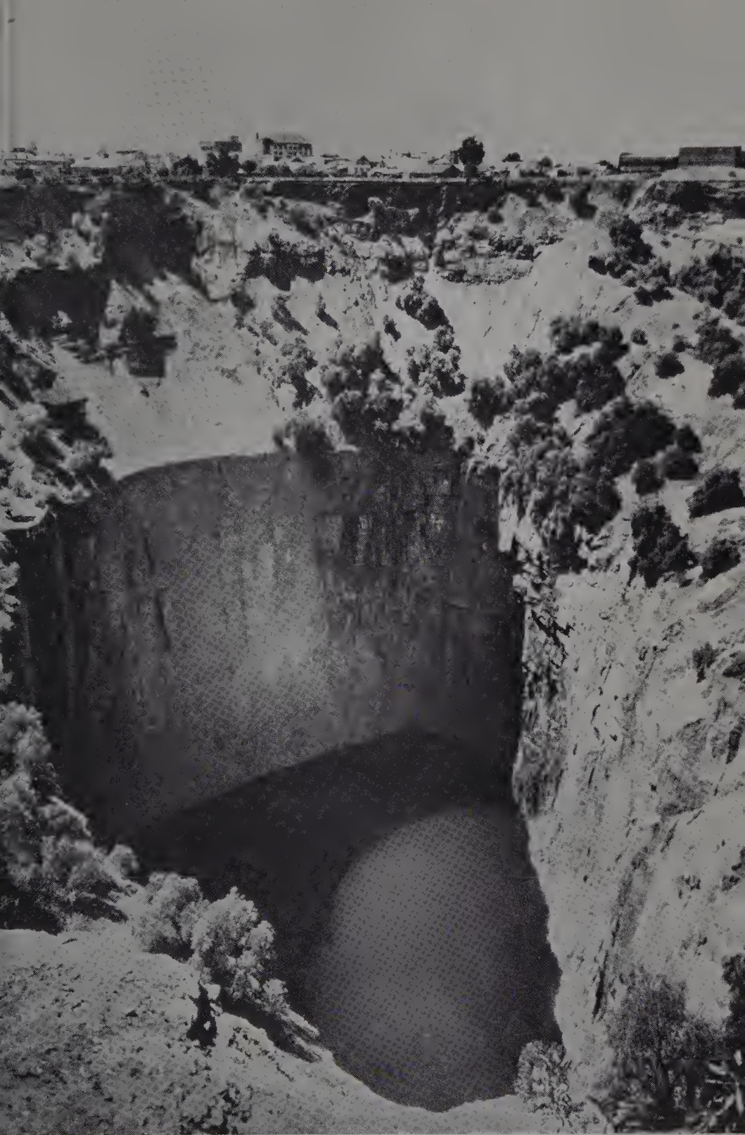
The 'Big Hole' at Kimberley. Kimberley Mine as it is to-day: a typical diamond pipe. Discovered in 1871 and finally abandoned in 1914, having reached a depth of 3,600 feet. Total production amounted to 14 million carats of diamond, valued at 47 million pounds. The surface area of the mine is 38 acres. See page 39.
