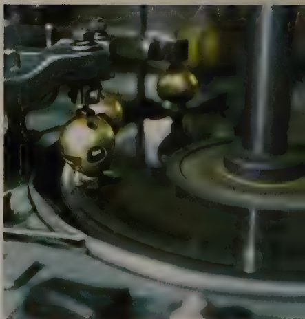
Faceting of diamond on horizontally rotating cutting wheel with the help of a dop.
