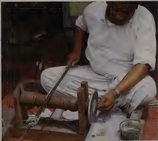
Gemstone cutting with vertically running wheel and fiddle-bow drive; Sri Lanka.
