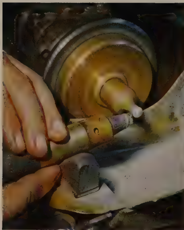
Two diamonds receive their raw shape for the brilliant cut by rubbing them against each other.
