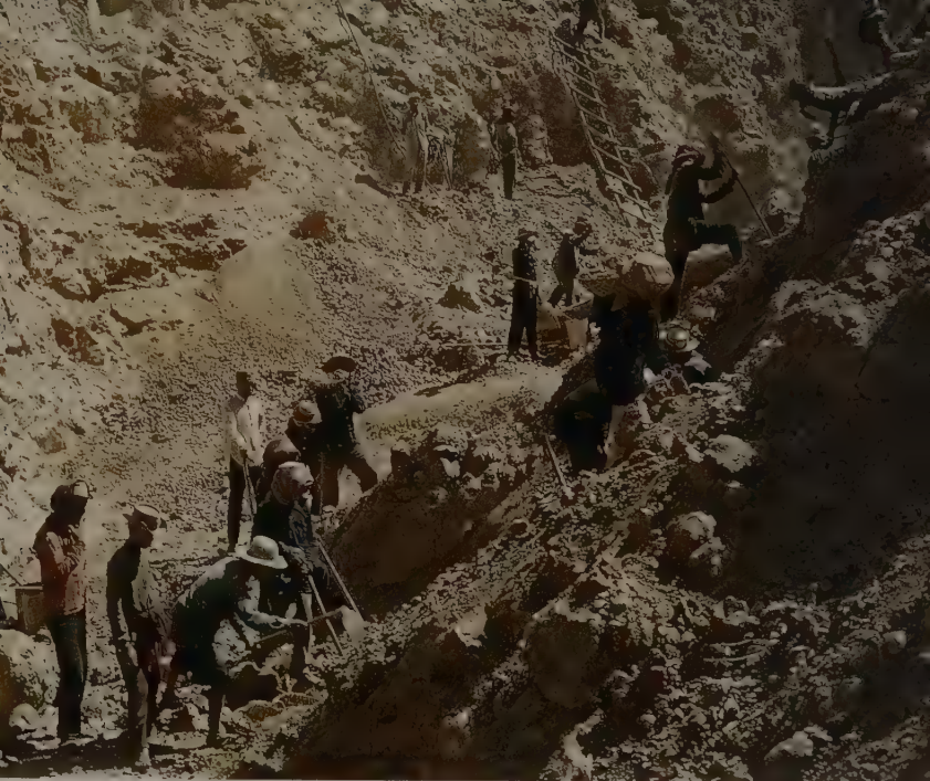
Fluorite mine near Chiang Mai/Thailand. Without using machines, the strongly weathered rocks are being loosened, carried off, and sorted.
