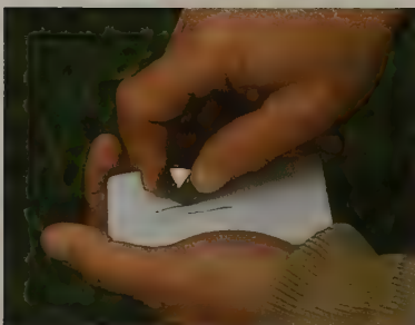
Streak test on a streak plate. The brassy yellow pyrite leaves a greenish-black streak of color.
