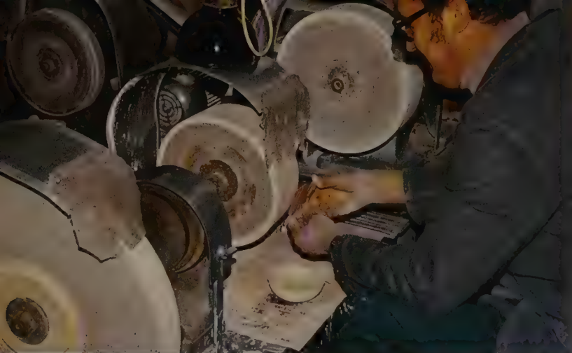
Polishing of agate on slowly rotating wheels without or with only a little cooling fluid.
