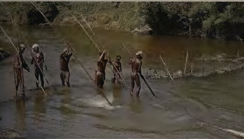
Loosening of gemstone-bearing sediment in a river; Sri Lanka
