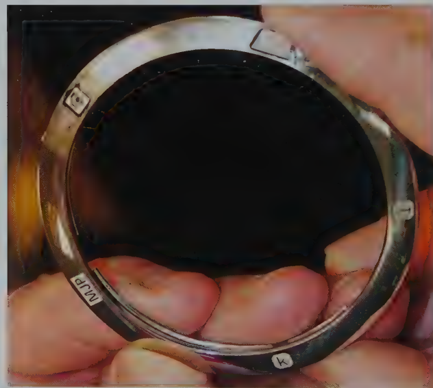
Example of a laser hallmark on palladium. (Photo: KW/courtesy of Birmingham Assay Office)
