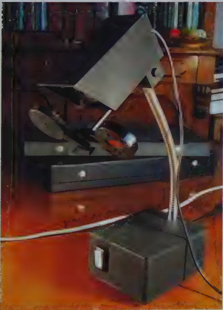
High intensity lamp with sodium filter and visual optics filter and fibre optic (designed by the author). (Photo: KW)
