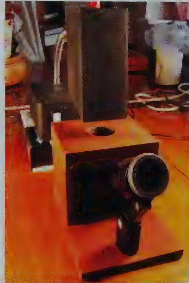
Crossed filter assembly (simple test for chromium content). (Photo: KW)
