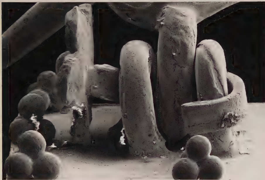
Above FIGURE 27 Solder seam on the back of the hoop of the ring from Tharros (no. 153). The scanning electron microscope photograph exaggerates the colour contrast.
