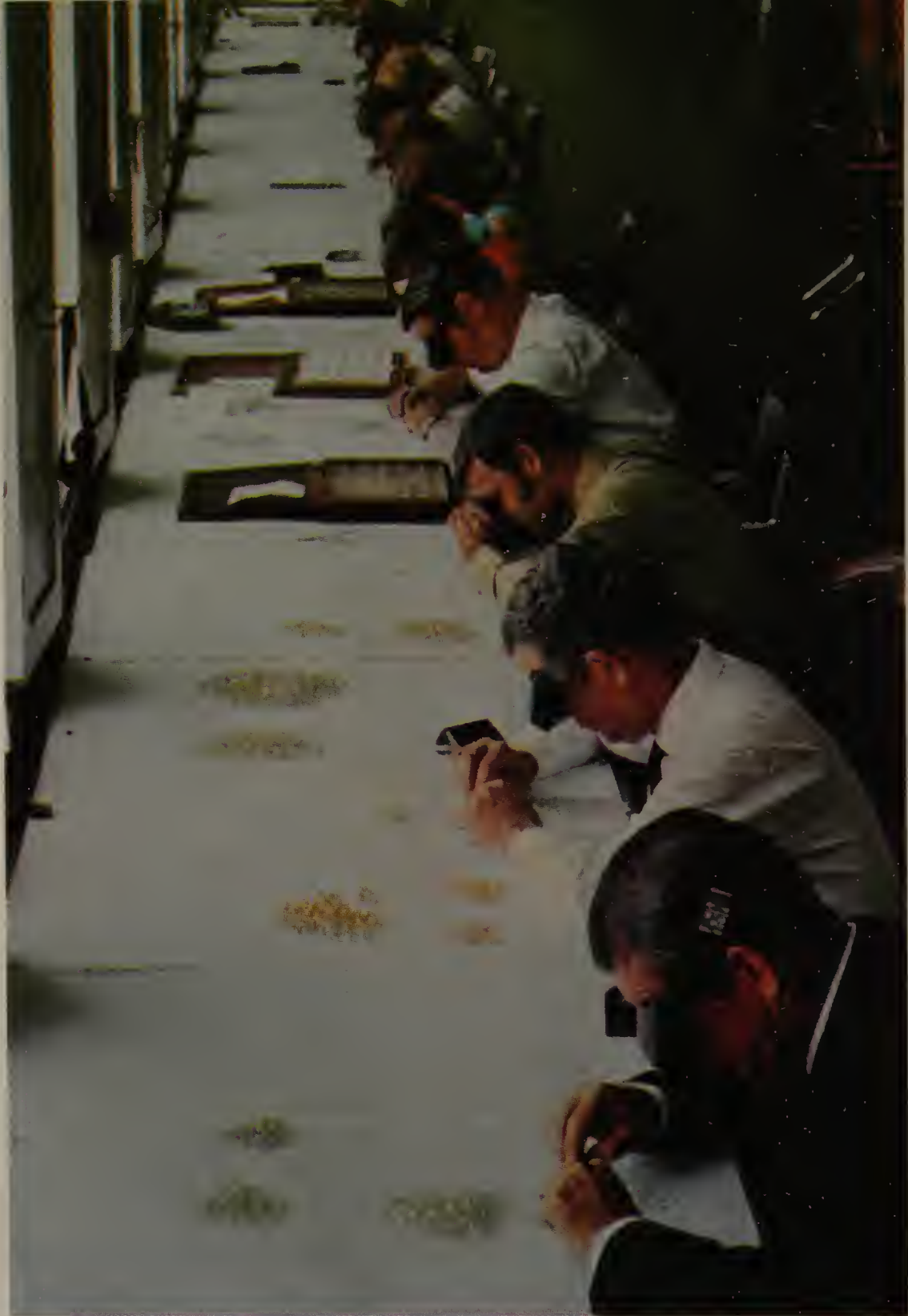
The heart of the De Beers system of 'sights' is the careful sorting into over two thousand grades (by size, shape, quality and colour) of rough diamond crystals. Note : Some diamond piles are yellowish.
