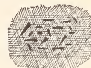
FIG. 4.—Cuneiform crystals in ruby and sapphire (enlarged 200 diameters).
