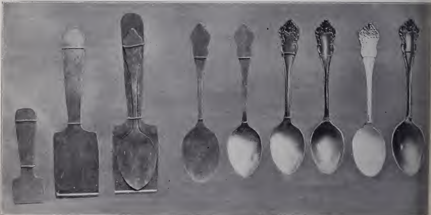
(1) BLANK. (2) ROLL. (3) PRESS-OUT. (4) ROUGH. (5 AND 6) STRIKE-UP. (7) POLISH. (8) SILVER PLATE. (9) HAND BURNISH.
