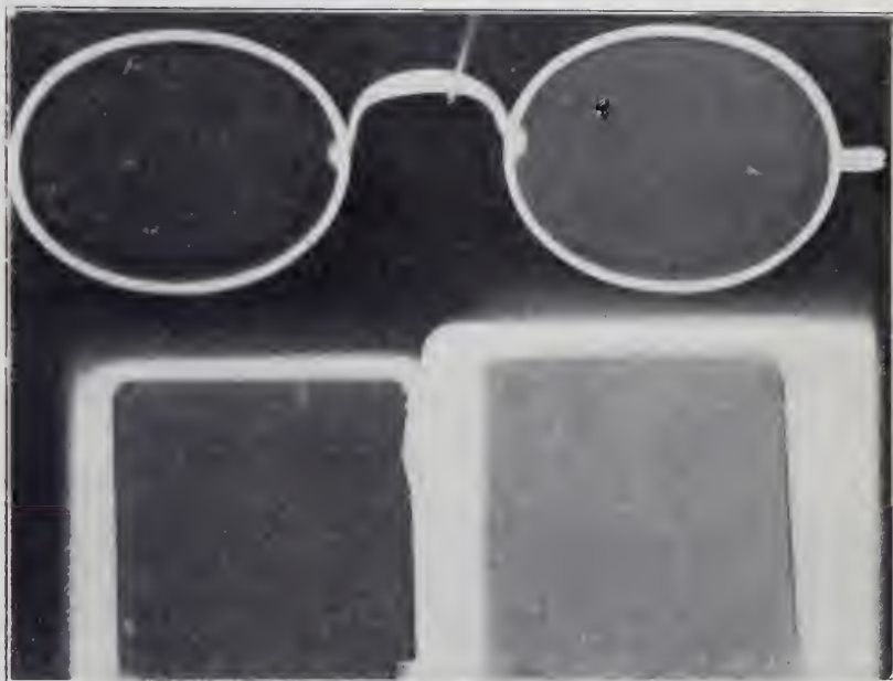
PHOTOGRAPH SHOWING TOTAL TRANSMISSION OF LIGHT BY "HEALTH RAY" GLASS.
