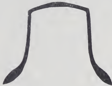
SECTION OF BELL SHOWING VARYING THICKNESS.
