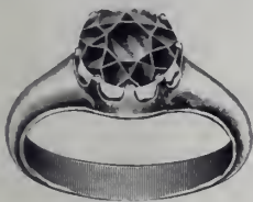
Tiffany ring as received with worn off claws. Stone cannot be reset, as it would be too low to look well and the point would come below the inner circle of ring. (See cut No. 2 of flat belcher.)
