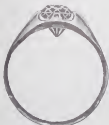
How the same ring looks when stone is reset without new claws. Stone is not secure and point is below inside of ring.
