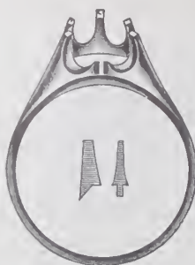
How we splice settings and solder in new claws; seams do not show and rings are as perfect as when originally made.
