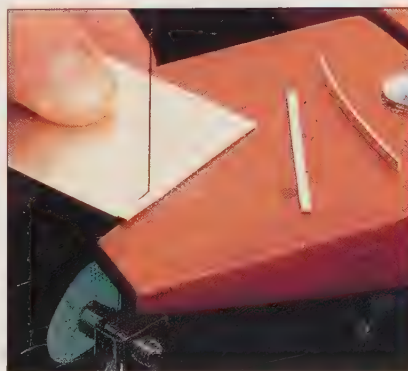
The bezel lengths are cut for the settings.
