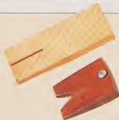
A pin that is suitable to fix to a transportable workbench (below) and an example of a permanent fixture to a bench (above).
