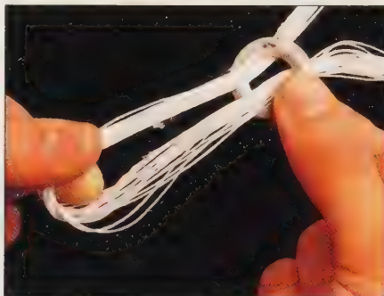
Polishing strings – use as many or as few as you need to reach difficult areas.
