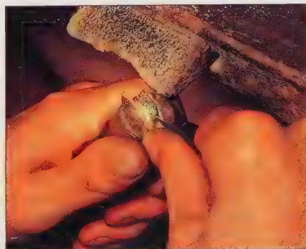
A half-round scorper is used to raise the grains round each diamond, and then the grains are pushed down with the beading tool.
