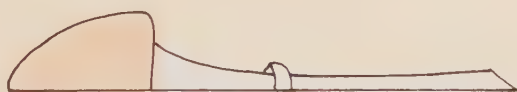
A straight graver is used for working on a flat or convex surface
