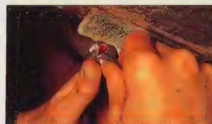
A pusher is used to rub the bezel onto the stone.
