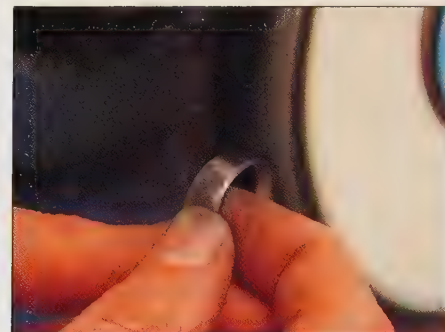
Polishing on an electric motor.
