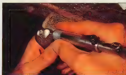
The setting is adjusted with burr in the pendant motor.
