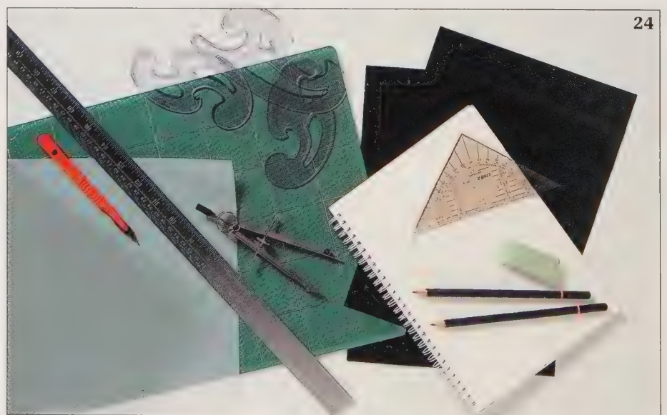
A pair of dividers and a steel rule graduated in inches and centimetres are invaluable to your work.
