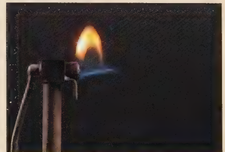
A small, hard flame, good for soldering very small areas.
