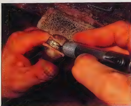
A pave setting. The holes are prepared to receive the stones with the drill on the pendant motor and then set in.
