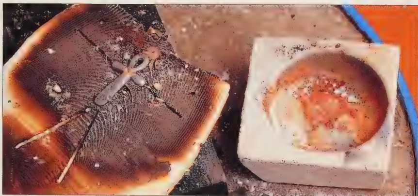
Molten silver is poured into the opening of the cuttlefish bone.
