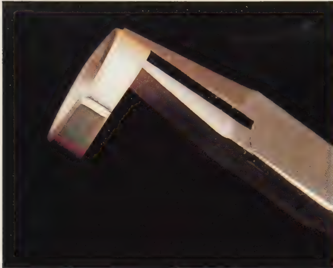
This joint is not correctly aligned for soldering. Even if the solder did run, the joint would need so much filing down that it would become very thin.
