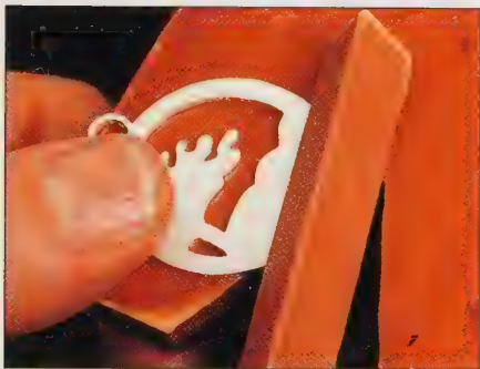
An emery stick is used to give a sanded finish.
