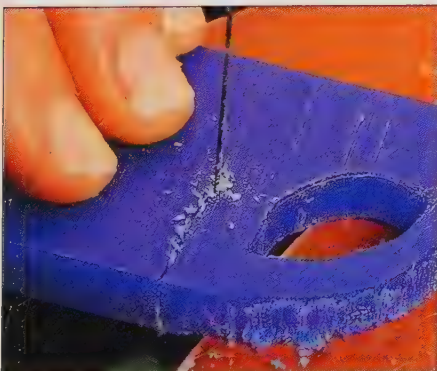
Modelling wax is cut with a piercing saw.
