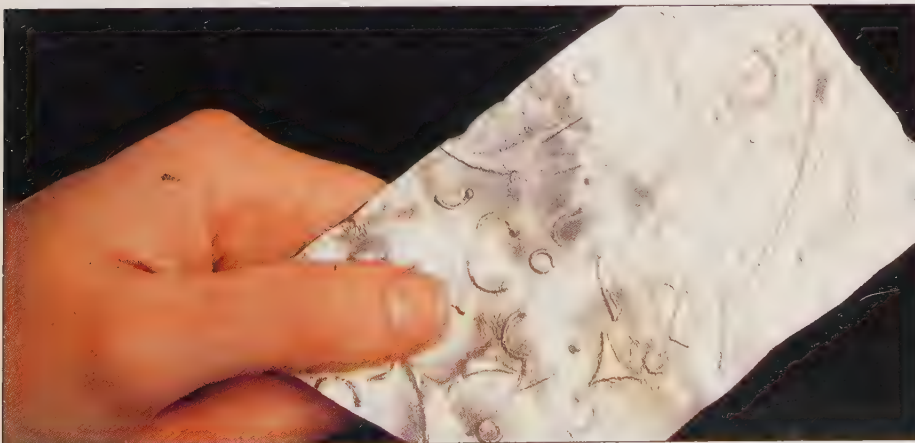
Reticulated silver sheet; the top half has been quenched and is ready for piercing.
