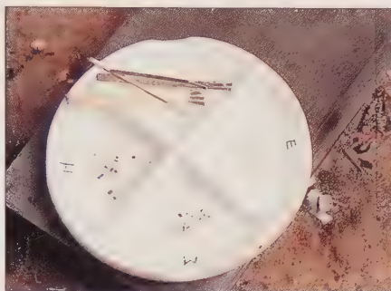
Keep a divided dish near the soldering area for strips and paillons of hard, medium and easy solder.
