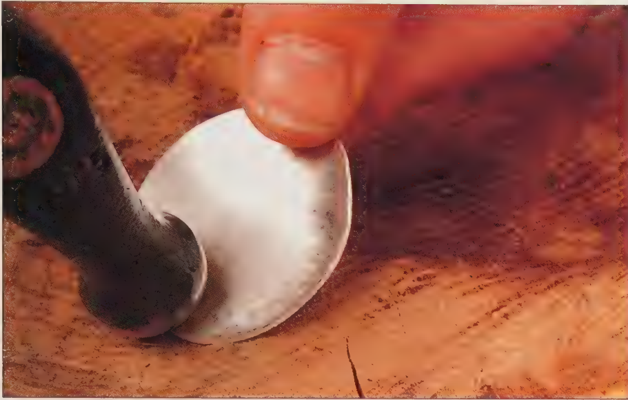
A silver disc is shaped on a wooden block.
