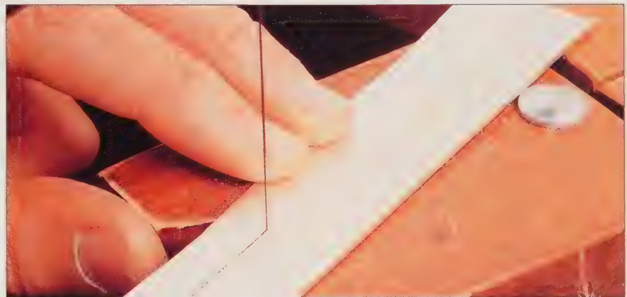
The outline is pierced after stop out has been removed.
