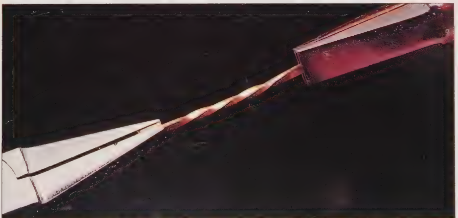
Square wire is twisted for chain links.
