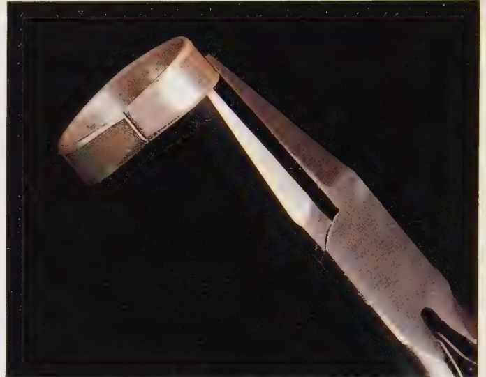
This joint is correctly aligned which will, therefore, allow the solder to flow easily.
