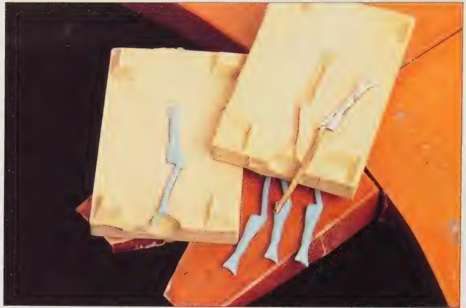
The rubber mould is formed around your original model and sprue. Here it is in two halves with some wax models, which have
