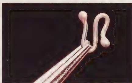
Wire for hook with both ends run up to make little balls.
