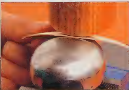
When you are shaping silver, keep the area being worked with the hammer or mallet in direct contact with the stake.
