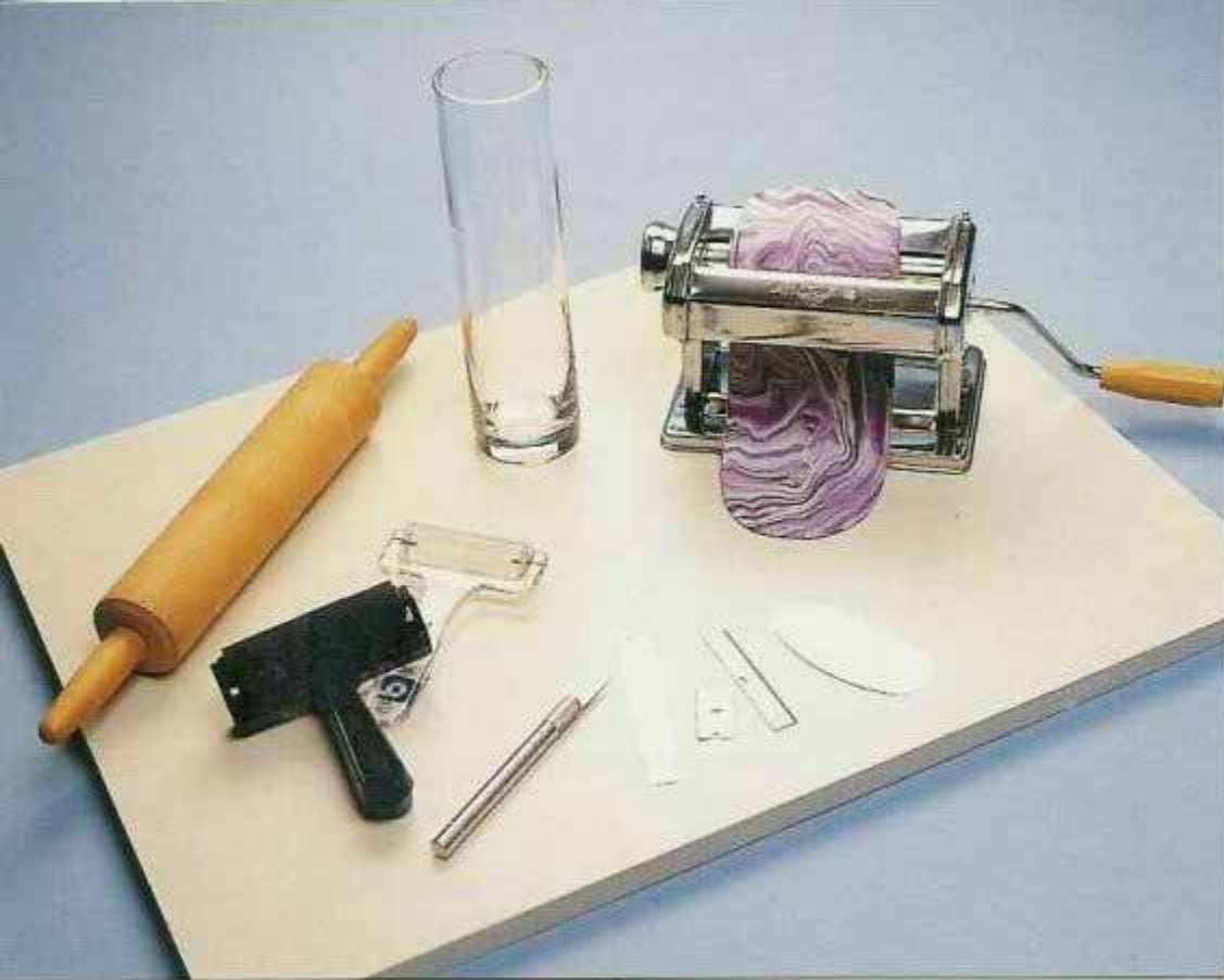
Arranged on a work surface are some examples of rolling tools: two types of brayers, a rolling pin, glass vase, and pasta machine. Next to the craft knife is an assortment of slicing blades (left to right): tissue slicing blade, single-edge razor blade, a wallpaper scraper blade, and a clay slicing tool.
