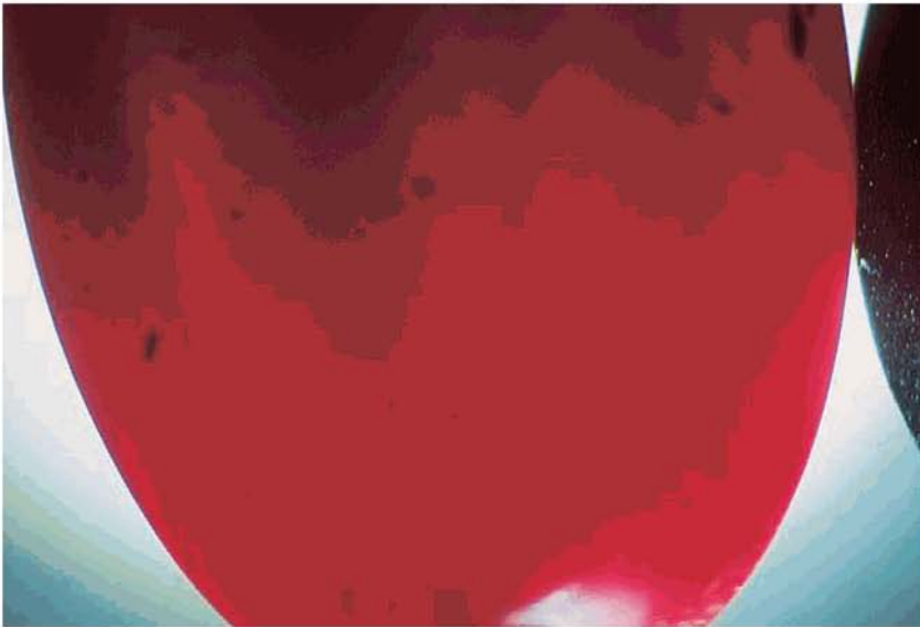
Figure 13.6 Detail of Bakelite ear-ring, viewed by transmitted light, showing faint elongated colour bands.
