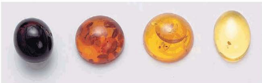
Figure 1.19 Baltic amber cabachons, showing the effects of progressive degrees of heat treatment. The palest bead is untreated.
