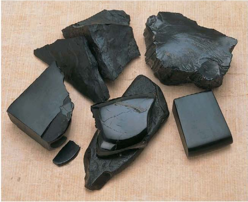
Figure 2.1 Various jets, clockwise from bottom: Whitby half polished on top of Whitby rough, Mexican half polished, Mexican rough, Ukrainian rough, Chinese polished.
