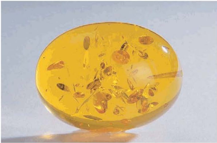
Figure 1.23 Plastic simulant with imitation stress fractures.
