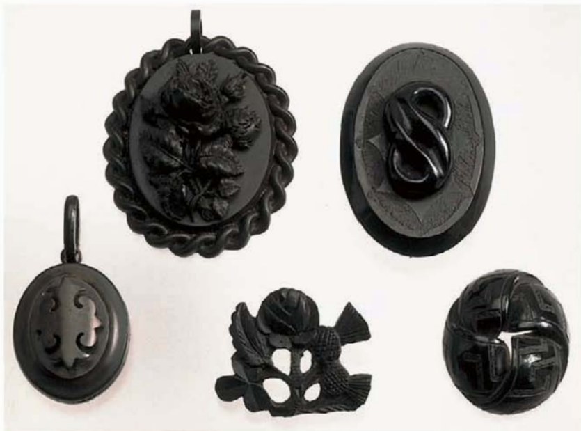
Figure 2.3 Jet and jet simulants. Top row: vulcanite, jet; bottom row: vulcanite, bog oak, jet.
