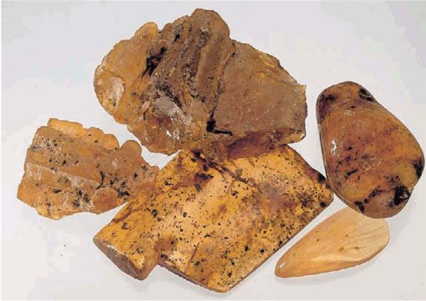
Figure 1.34 Pieces of rough and polished copal. Top, left and middle: South American copal; right: New Zealand kauri; bottom right, Dominican copal.
