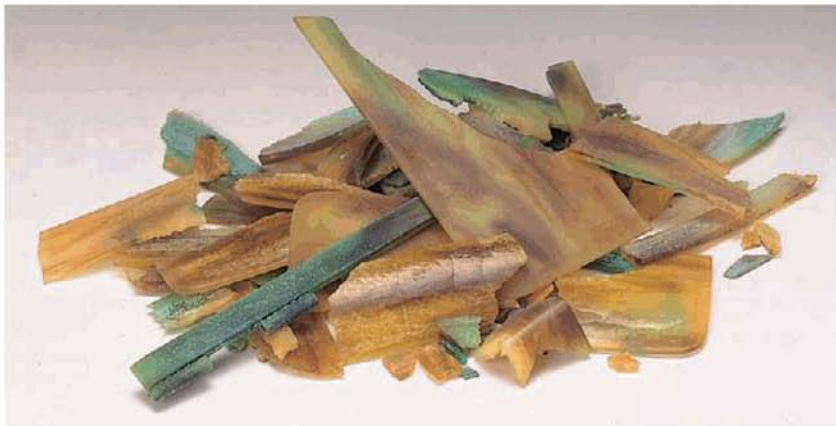
Figure 13.3 Degraded celluloid box that once imitated tortoiseshell.
