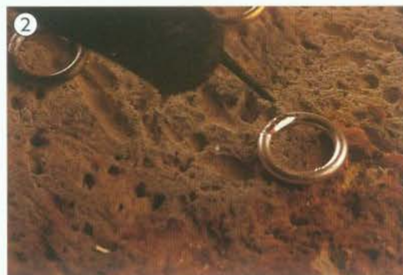
2 Solder is brought into contact just as the work reaches soldering temperature.
