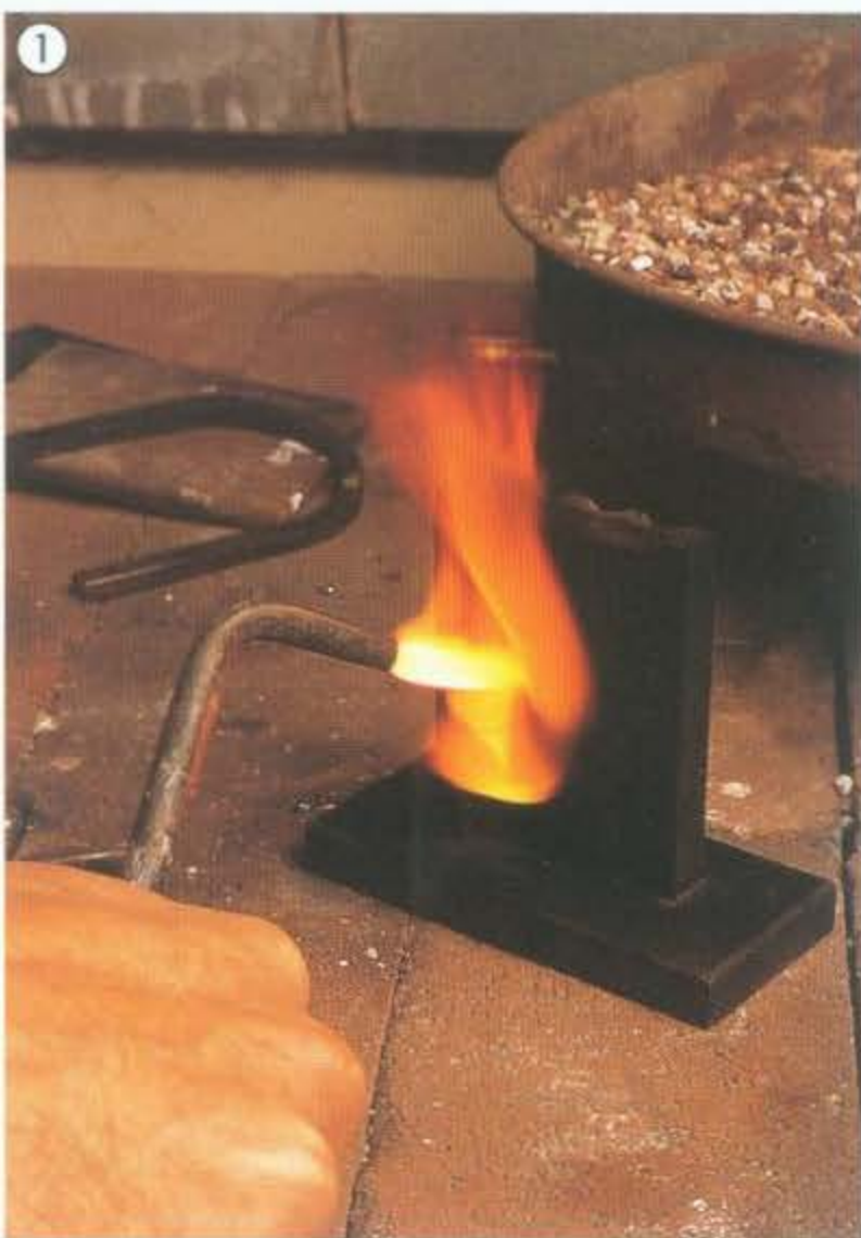
1 Coat the ingot mold with soot; this will create a reducing (purifying) environment.
