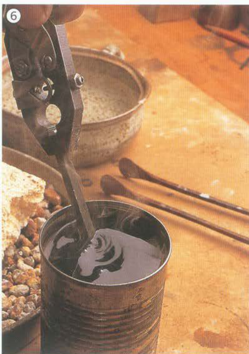
5-6 Heat the lower half of the tool to a bright red ... and quench it in oil.
