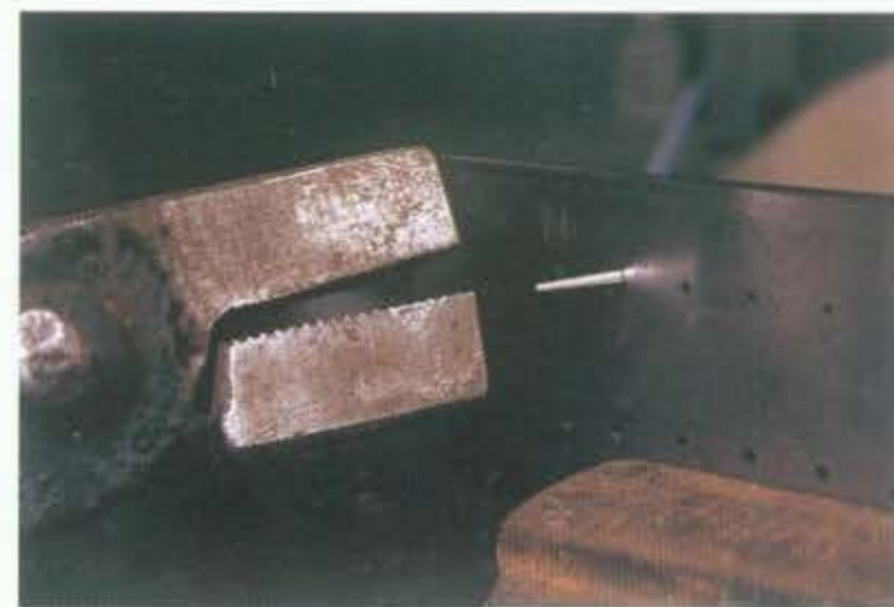
Draw tongs pull a wire through tapered holes of decreasing size in a drawplate.
