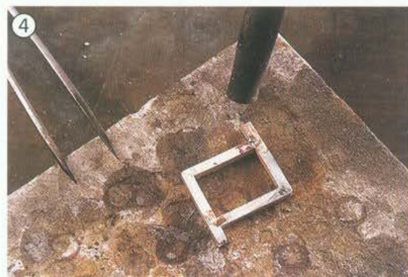
3-4 File until the two vertical legs are identical. Set the two pieces together; note that the sides are automatically parallel.
