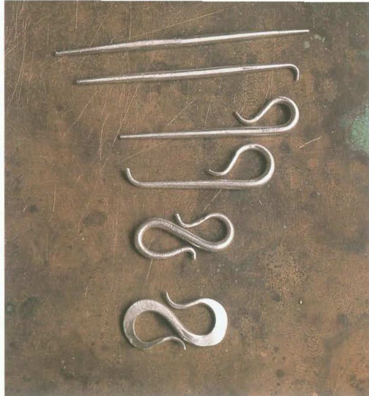
The steps in making an S-hook.
