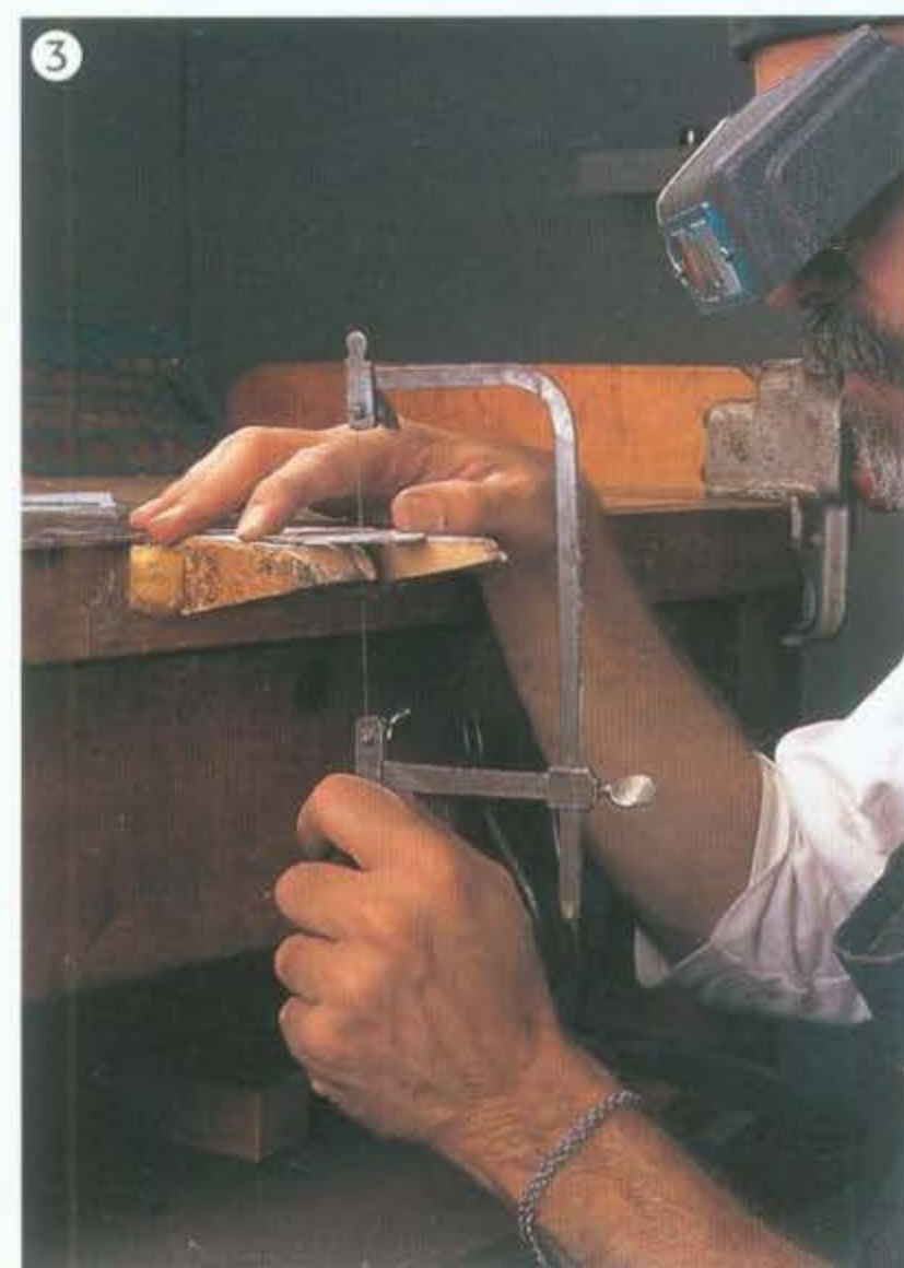
3 The proper posture for sawing: Keep the blade vertical.
