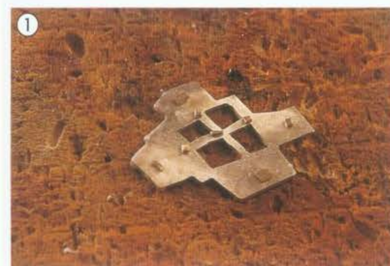
1 In sweat soldering, start by melting solder onto the back of one piece...
