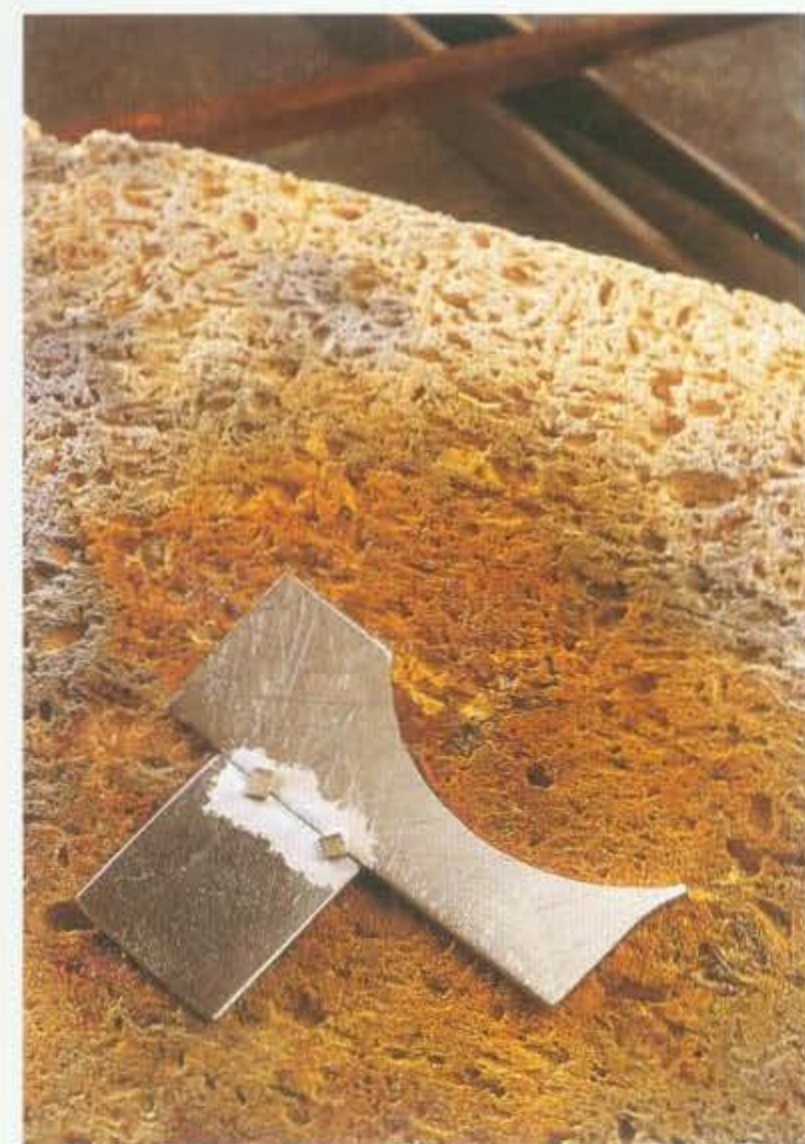
Chips of solder span a fluxed joint.
