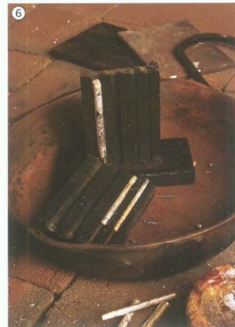
6 Finished wire ingots. These can be rolled or forged to make wire.
