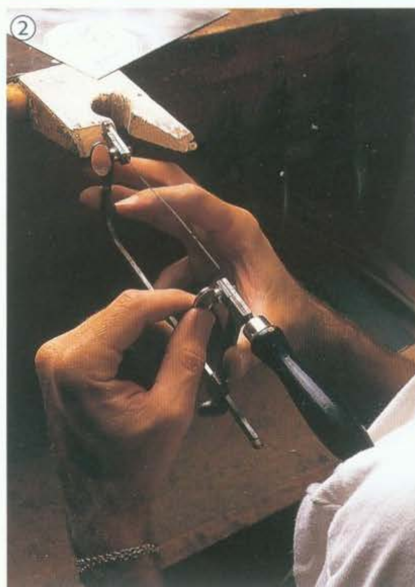
2 Support the saw frame against your chest as you insert the blade.
