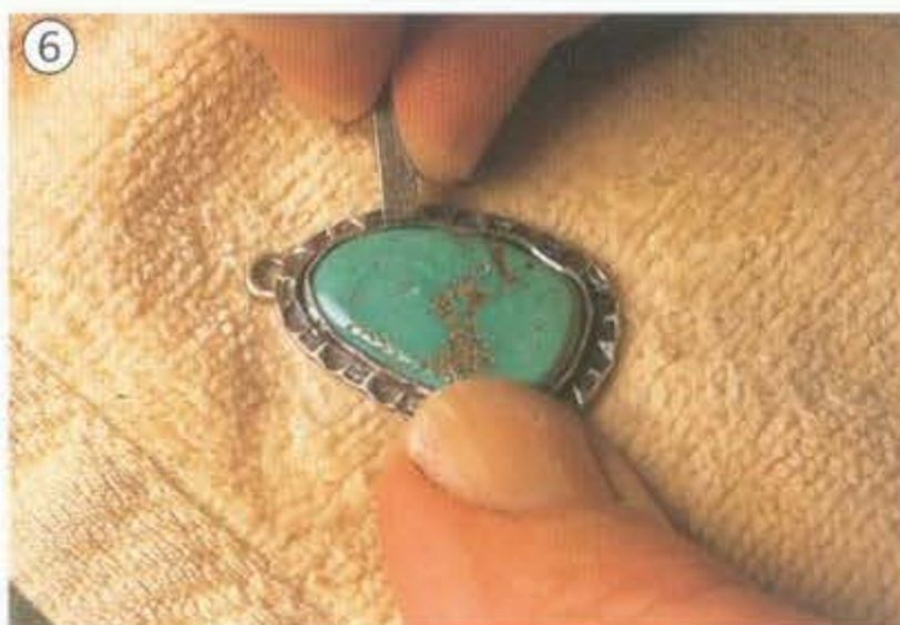
6 Working side-to-side, use a bezel pusher to press the bezel against the stone.
