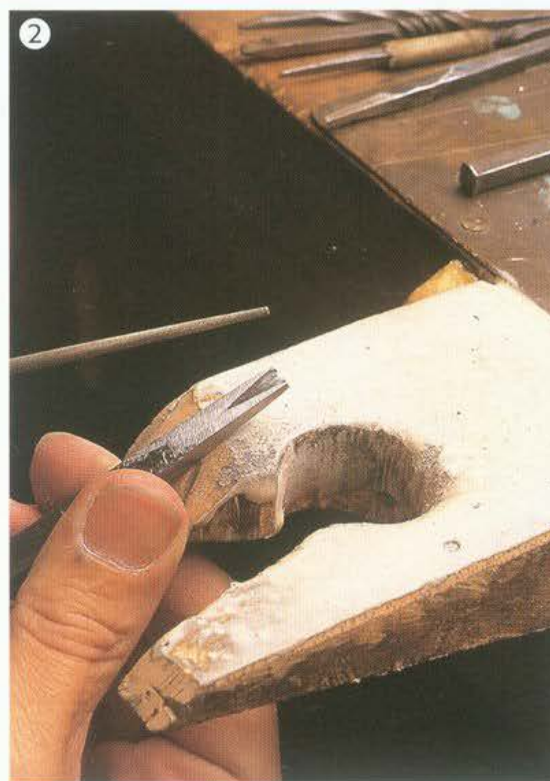
2 Create the intended shape in the end of the rod with a saw and files.
