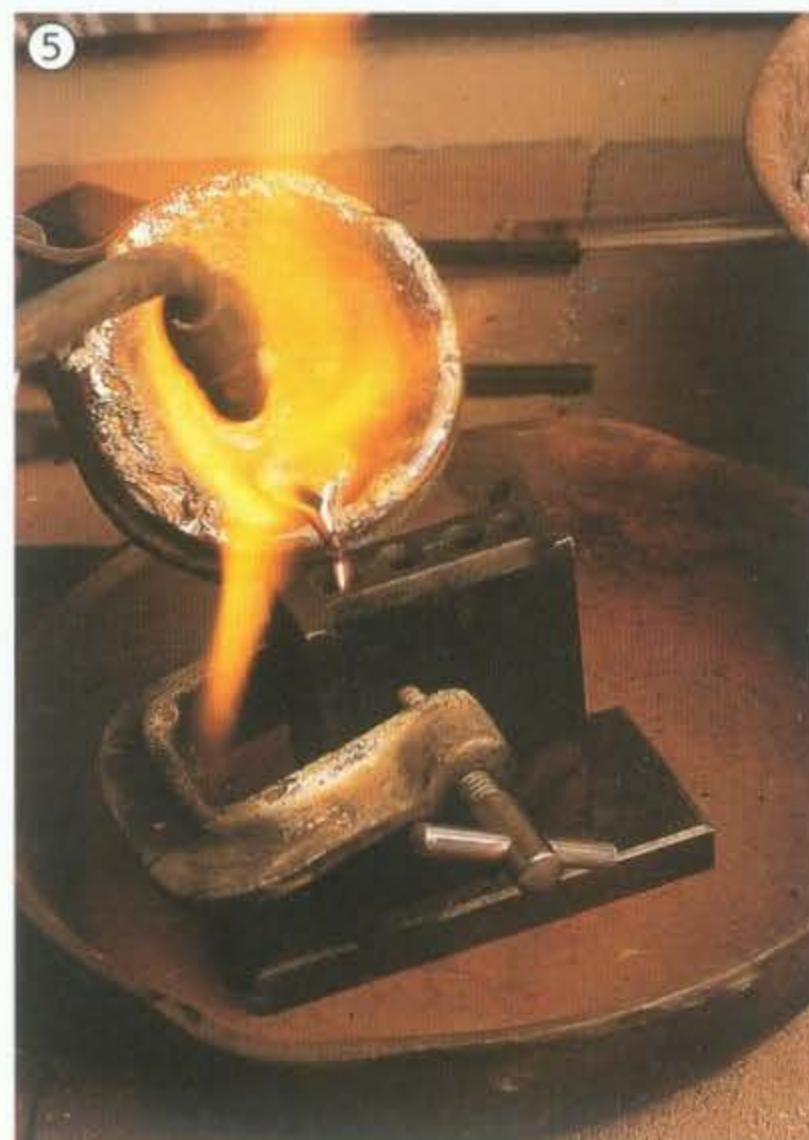
5 Pouring into a wire mold.
