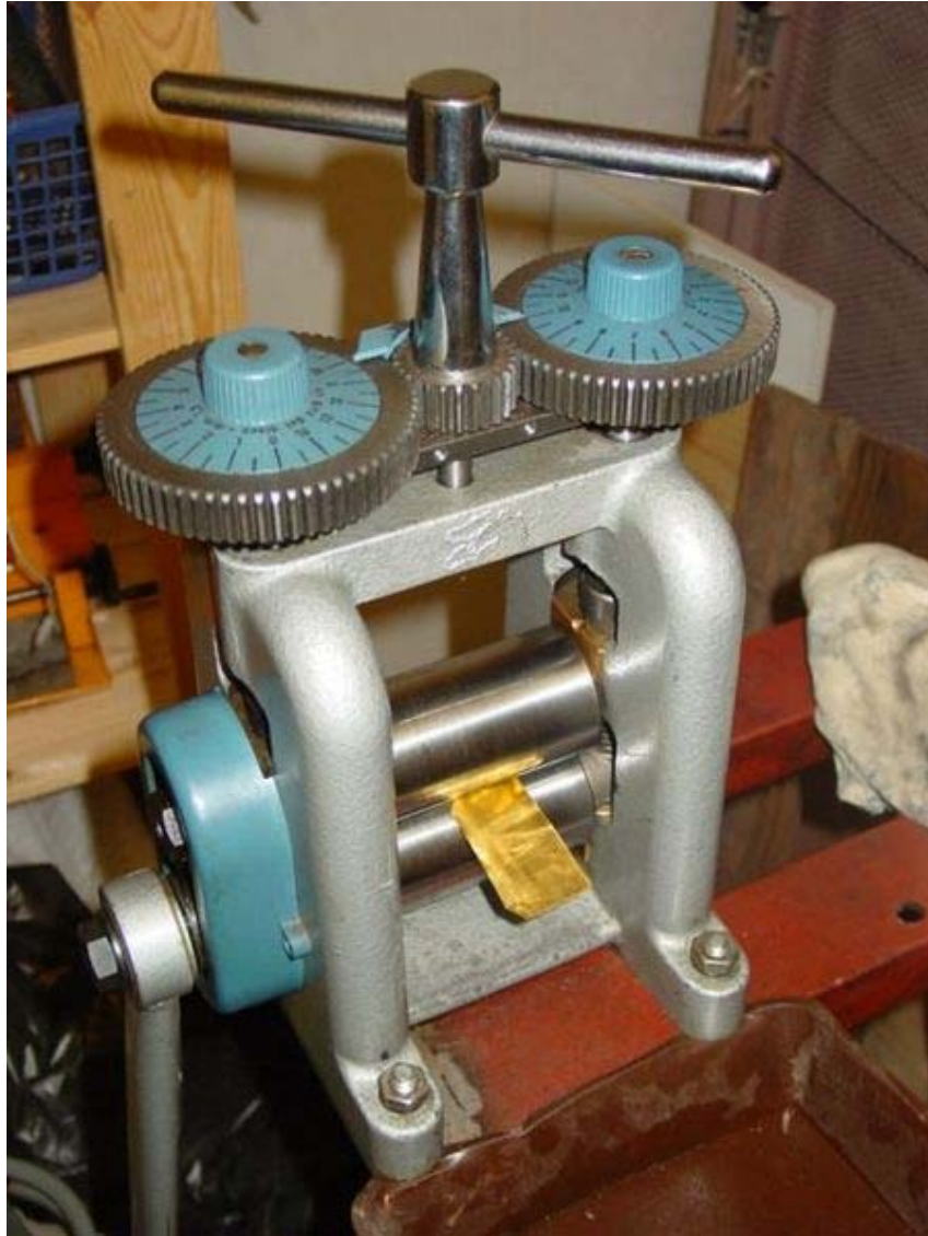
Rolling mill for cold rolling metal sheet like this piece of brass sheet
