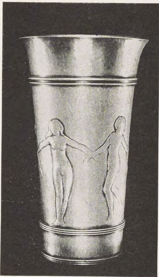
FIG. 88. SILVER CUP, HAMMERED UP FROM CIRCULAR SHEET. IN PROCESS OF BEING CHASED. BY AUTHOR
