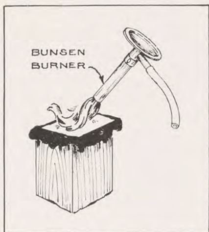
FIG. 67. USING THE BUNSEN BURNER FOR HEATING THE PITCH
