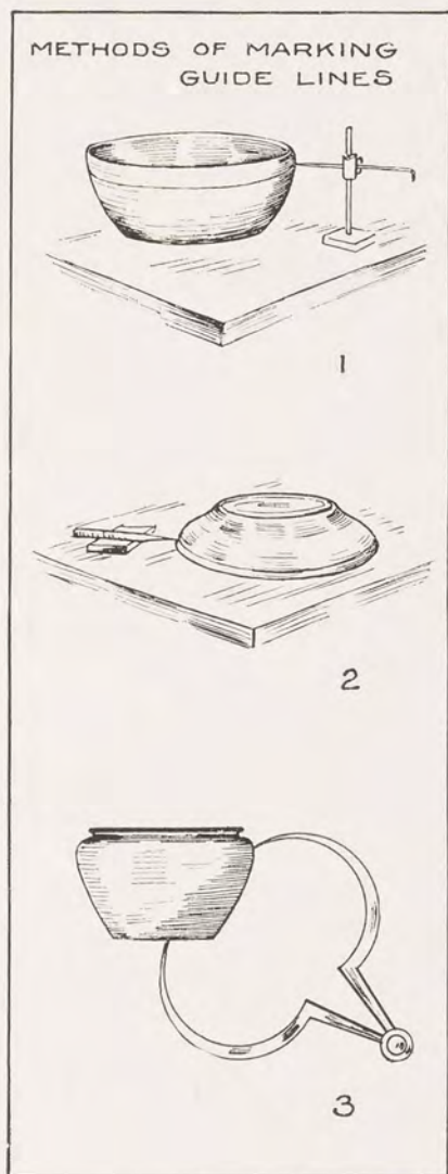
FIG. 142. DIFFERENT METHODS OF GAGING OR MARKING A LINE
