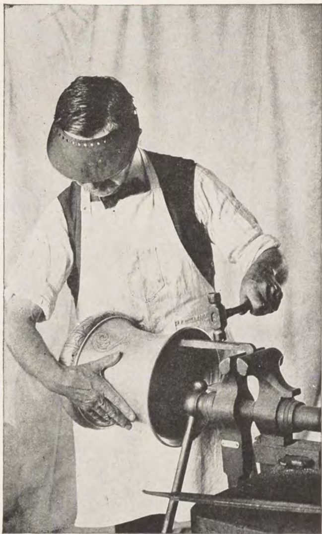
FIG. 87. RAISING ORNAMENTS ON VASE BY THE USE OF THE SNARLING IRON By courtesy of The Gorham Co., New York
