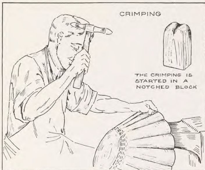
FIG. 139. RAISING A VESSEL WHICH FIRST HAS BEEN CRIMPED
