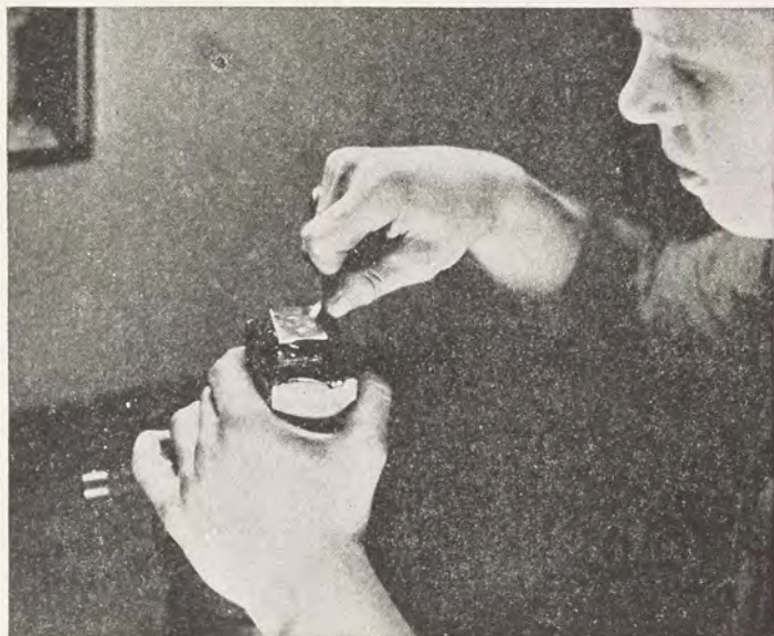
FIG. 51. WORK BEING CARVED. ATTACHED TO PITCH BLOCK AND HELD IN THE ENGRAVER'S BALL
