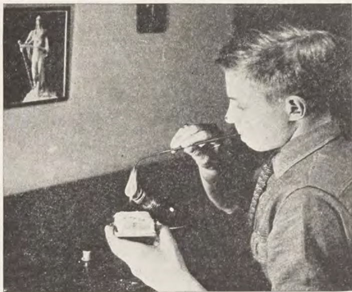
FIG. 33. SOLDERING WITH ALCOHOL LAMP
