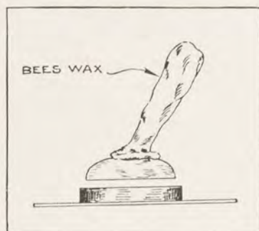
FIG. 40. FITTING STONE INTO BEZEL
