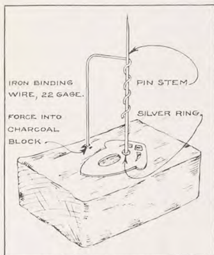
FIG. 58. METHOD OF HOLDING PIN STEM IN PLACE WHILE SOLDERING
