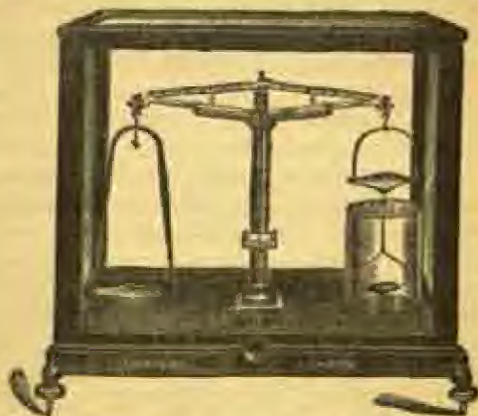
Fig. 1.—Balance for hydrostatic weighing in determining the specific gravity of gem-stones
