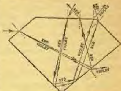
Fig. 16.—Splitting up of light in a brilliant-cut diamond: refraction and internal total reflection
