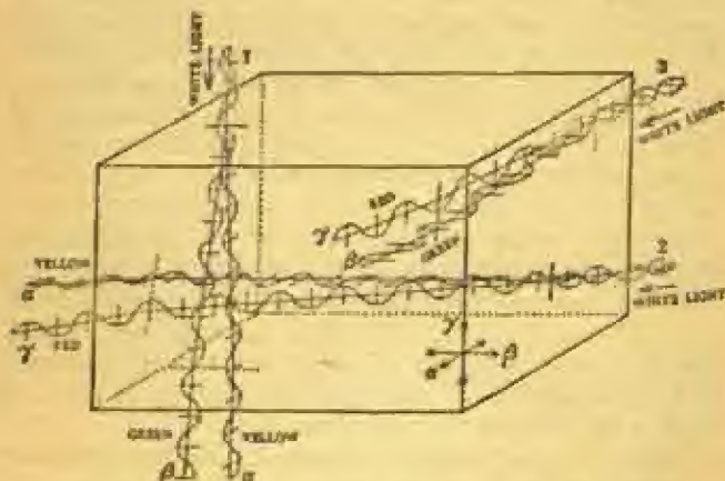
Fig. 21.—Pleochroism. Adventures of white light in a coloured, optically biaxial crystal. A box of conjuring tricks
