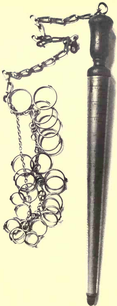
THE "ALLEN RING GAUGE" Generally used in the United States for measuring accurately the size of the ring required to fit a given finger
