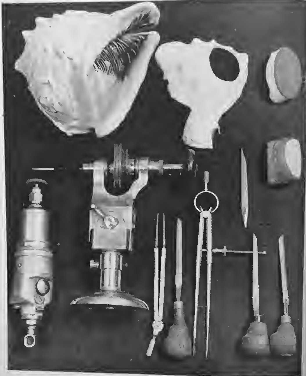
Articles used in cameo cutting. Whole shell at top, back of shell removed, buffer and cameo blank mounted. At bottom are shown an air tool, graver blades and other mentioned articles.
