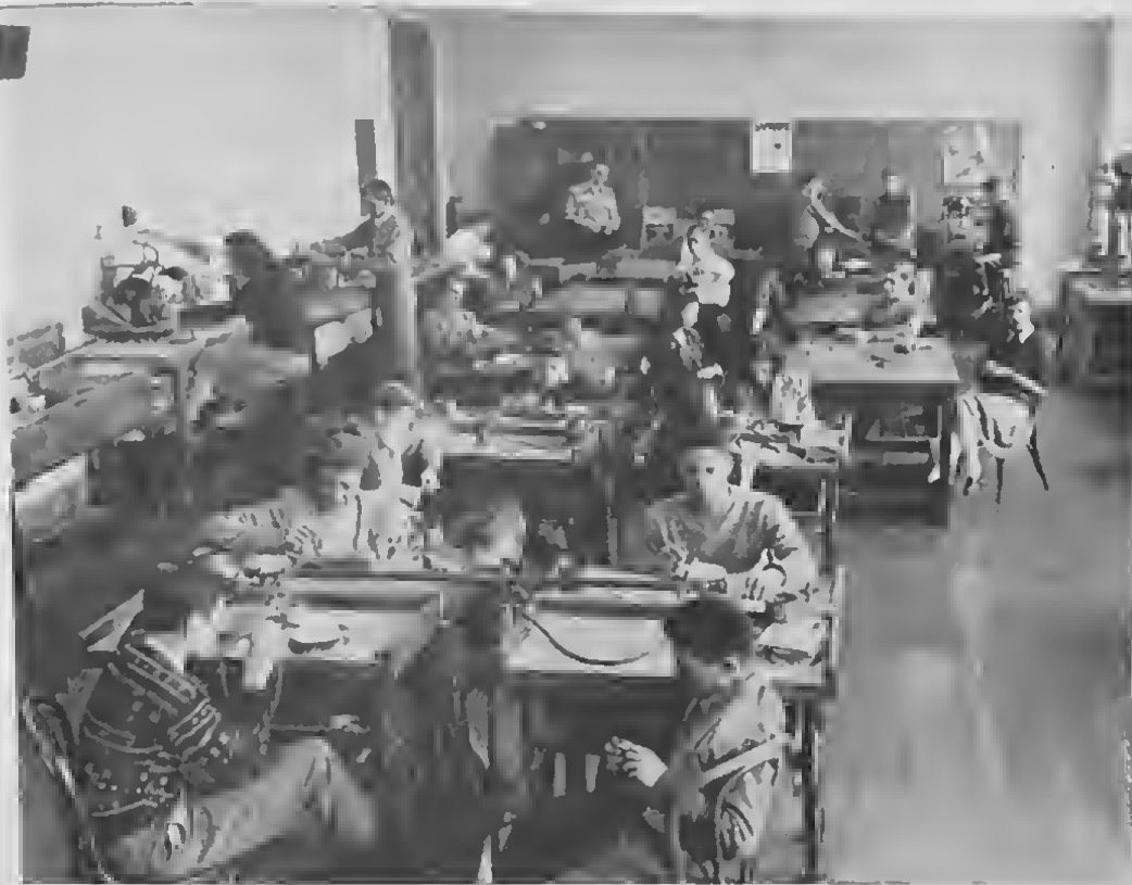
View of Jewelry and Gem Cutting class at Woodrow Wilson High School, Washington, D. C. Girl at left is grinding a gem. Boy at the back (white shirt) is working at a flat lap. Boy at right (rear) is drilling a pendant. Students in the foreground are working at soldering benches. Note that about a third of the class is girls. This is a very popular course. Instituted by Mr. Baxter in 1935, it now requires sessions for five groups daily.
