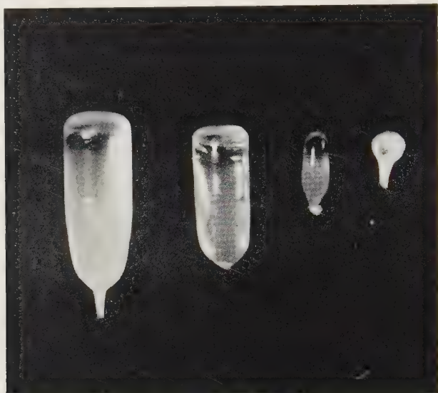
Figure 76 Stages of boule growth.
