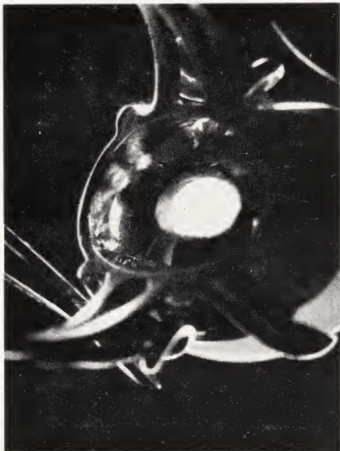
Figure 132 Color-enhanced jadeite. The coloring agent appears as an arc of gray at the left side of the opening.
