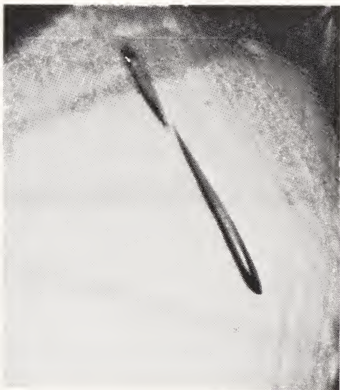
Figure 117 Greatly elongated gas bubbles in molded glass.
