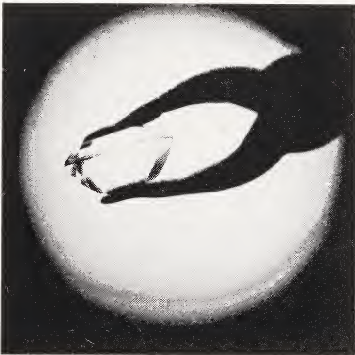
Figure 42 Cement layer on a triplet immersed in water
