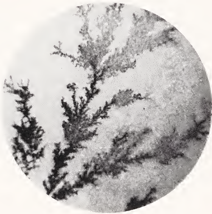
Figure 69 Moss-like arrangement of manganese oxide in moss agate quartz.
