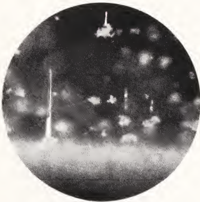
Bread crumb inclusions and two-phase spicules found in synthetic quartz.
