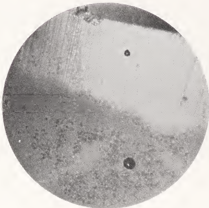
Figure 102 Slightly angular gas bubbles in synthetic spinel.
