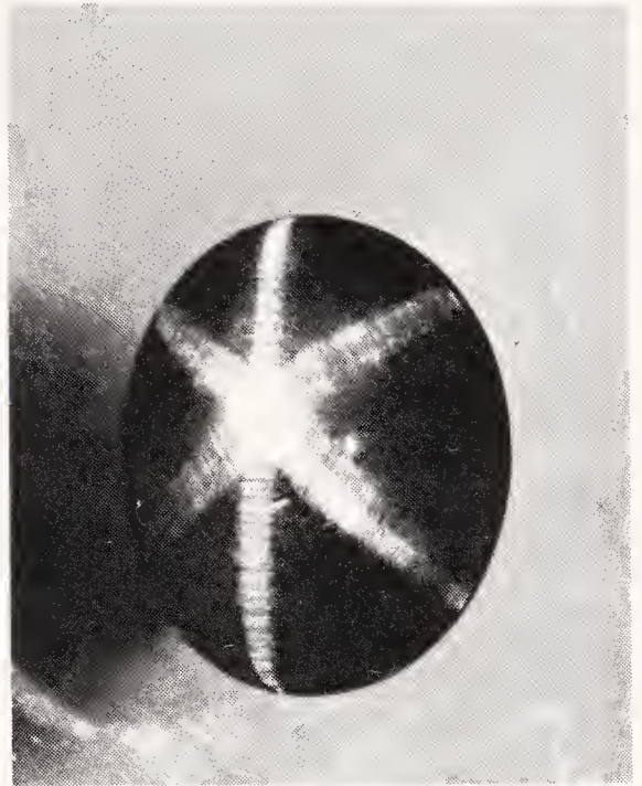
Figure 176 A synthetic sapphire backed by lined metal to simulate a natural star.
