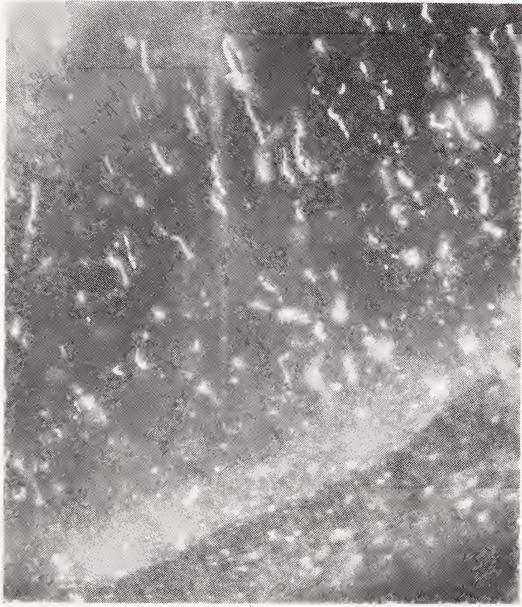
Figure 99 Thready or tubular inclusions in synthetic spinel
