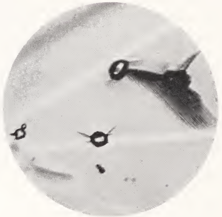
Figure 46 Included zircon crystals sur- rounded by a "halo" of black fractures in natural corundum
