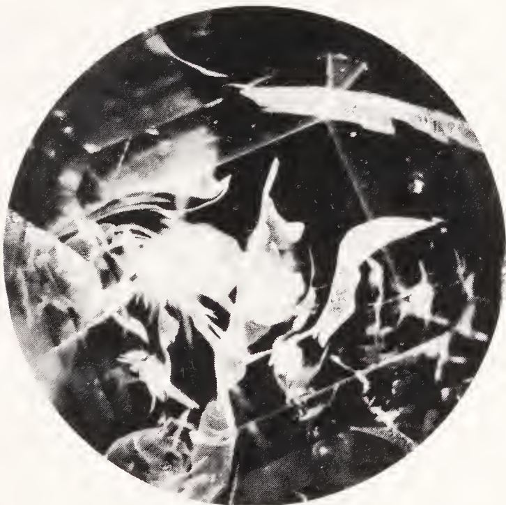
Figure 158 Veillike inclusions in a flux-grown synthetic emerald.
