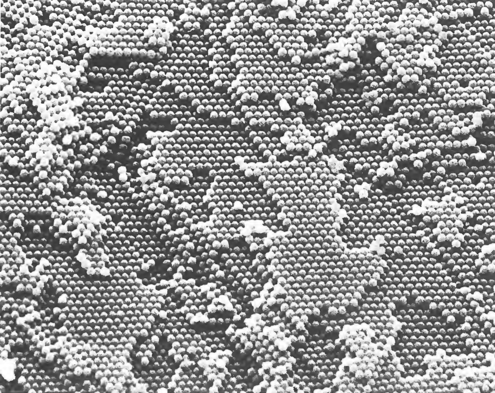
Fig. 6.3. Electron microscope photographs showing that opals are made up of tiny spheres of silica stacked in a regular arrangement.
