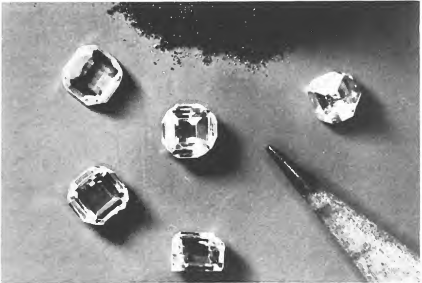
Fig. 4.8. 1-carat synthetic diamond grown by Robert Wentorf of GE, together with the graphite used as the starting material.
