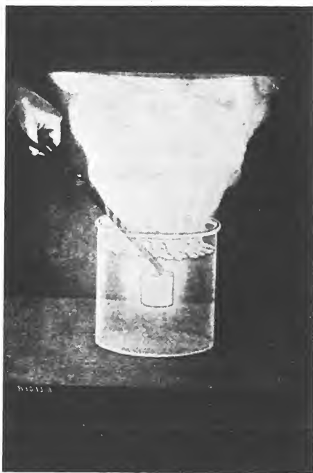
Fig. 4.2. (a) Moissan's 'Electric Furnace' with high temperature discharge. (b) Moissan's method of quenching a melt of carbon dissolved in iron by plunging into water.
