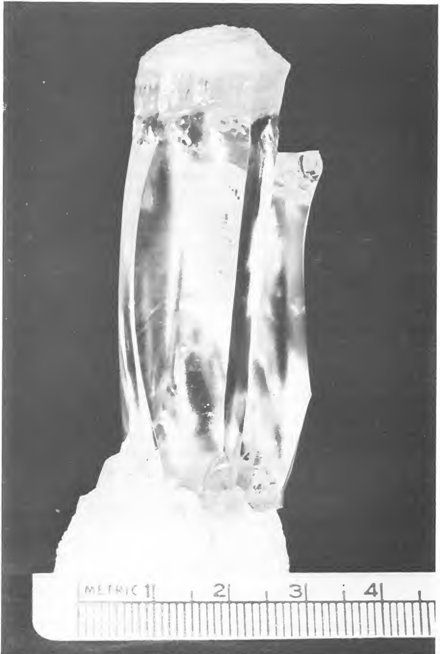
Fig. 5.5. Crystal of eubic zirconia grown by skull melting.
