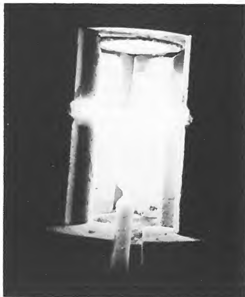
Fig. 2.5. (a) A line of production furnaces from the Djeva factory in Monthey, Switzerland. (b) Interior of a flame fusion furnace used for ruby production.
